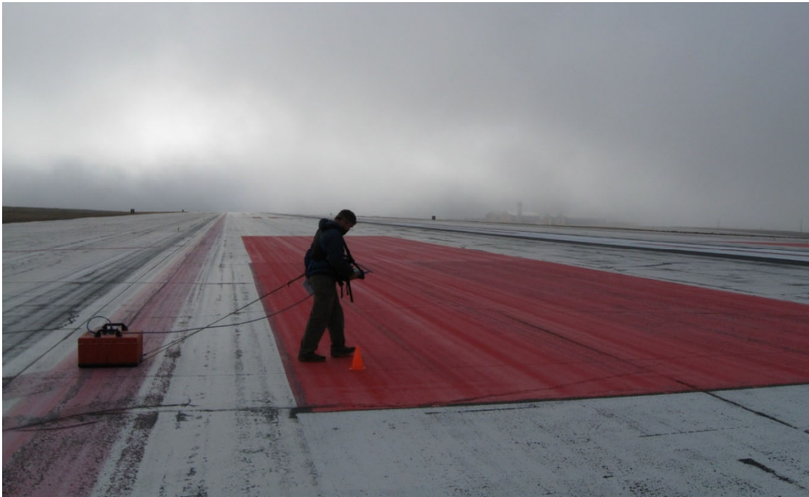
Figure 3-7 200 MHz antenna pulled over an airfield embankment.
