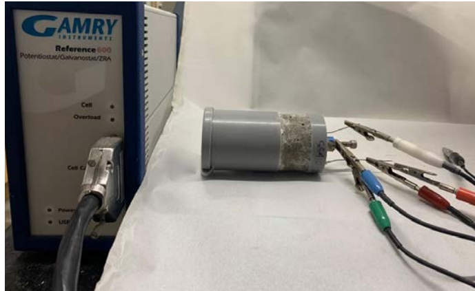
Figure 3.17: EIS measurement on UNS S41000 specimen labeled as B-I. Counter-electrode (embedded titanium mesh), reference electrode (embedded titanium wire), and working electrode (steel reinforcement bar).
