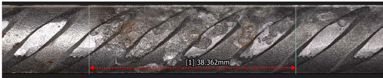
Figure 4.2: Optical image of plane measurement of the length of the anode in steel reinforcement.
