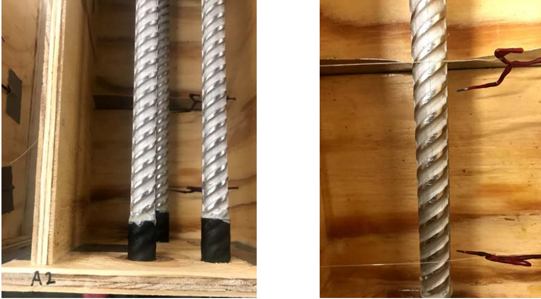
Figure 3.26: Experimental setup of reference electrodes.
