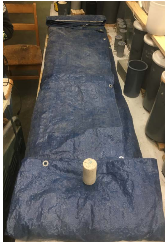
Figure 3.6: Concrete specimens with and without a tarp. Tarp usually covering the specimens was normally in place to avoid moisture evaporation and removed temporarily to take measurements.
