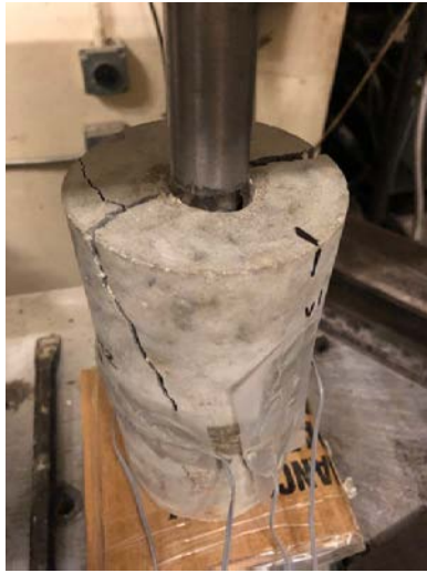
Figure 4.6: Extreme localized corrosion experimental results showing (a) concrete cracks, and (b) failure locations at the concrete cover. The red lines around the lead plug represent the concrete cover thickness at different locations ranging between 1.358 in and 1.595 in.
