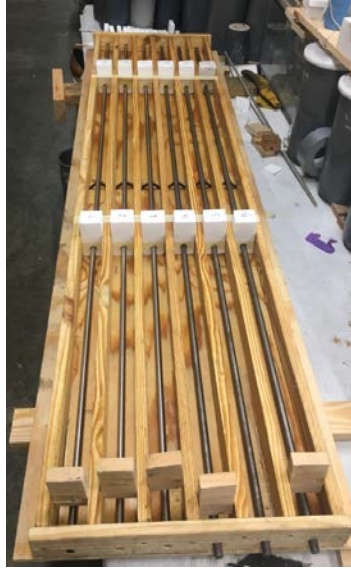
Figure 3.2: Wood mold coated with a mold release agent. Temporary polystyrene foam and 3D printed spacers were in place to implement the casting sequence to keep the concrete cover uniform.
