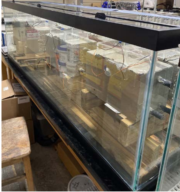
Figure 3.30: Specimens with concrete deficiencies in enclosed glass container.
