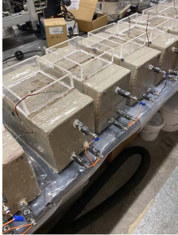
Figure 3.29: Specimens with concrete deficiencies. (a) Top view after acrylic reservoirs were installed; (b) preparation procedure prior to testing finished, two layers of epoxy were used to coat specimens and electrical connections. Circuit with 10-ohm resistor between anode and cathodes.
