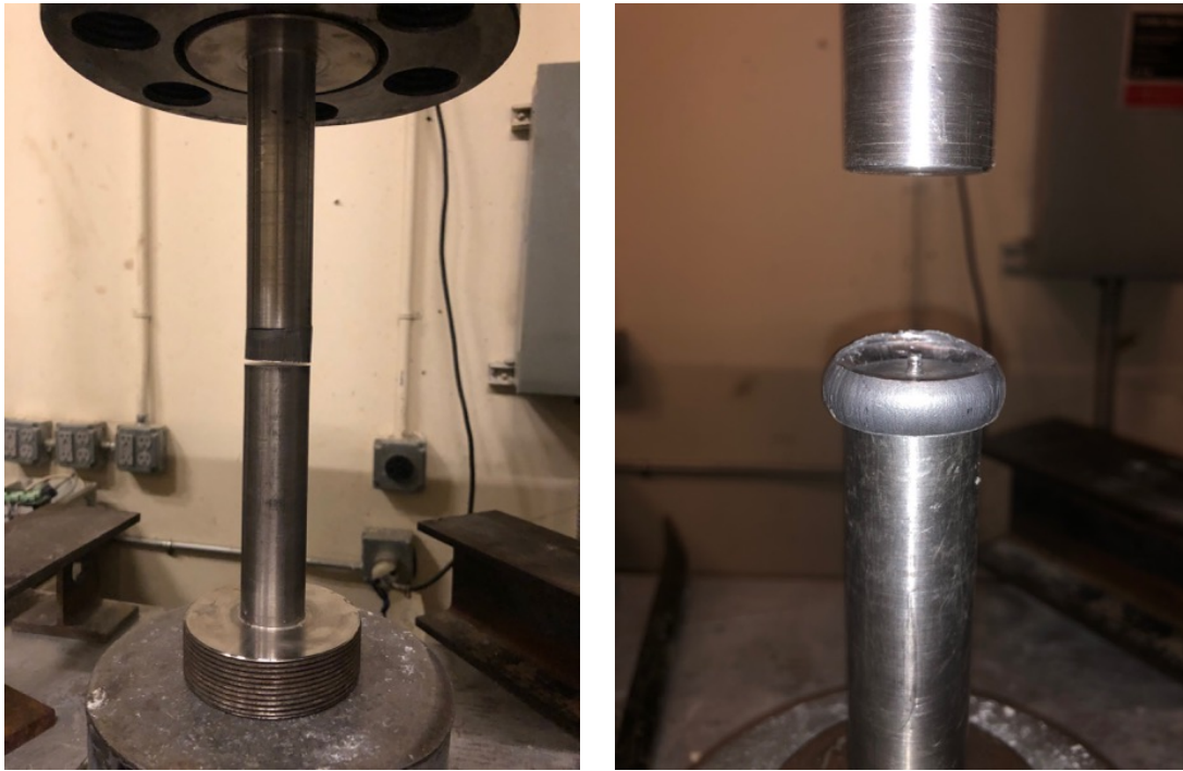
Figure 4.9: (a) Initial lead sample and (b) deflected shape of lead calibration.
