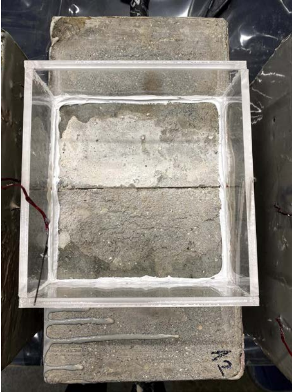
Figure 3.29: Specimens with concrete deficiencies. (a) Top view after acrylic reservoirs were installed; (b) preparation procedure prior to testing finished, two layers of epoxy were used to coat specimens and electrical connections. Circuit with 10-ohm resistor between anode and cathodes.
