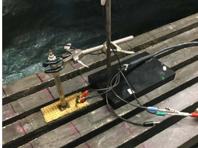
Figure 3.10: EIS measurement on specimen CS01. Counter-electrode (titanium mesh), reference electrode (SCE), and electrical junction device (yellow sponge).
