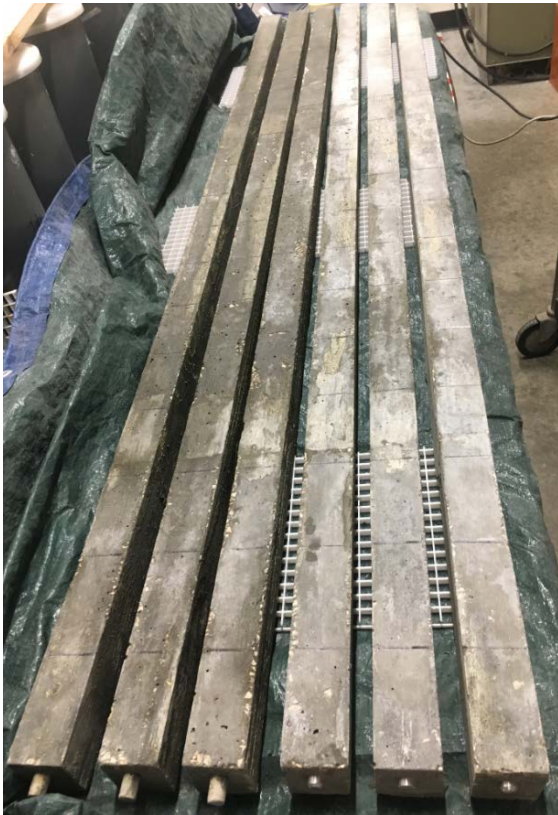
Figure 3.6: Concrete specimens with and without a tarp. Tarp usually covering the specimens was normally in place to avoid moisture evaporation and removed temporarily to take measurements.
