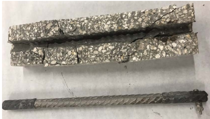
Figure 3.22: Steel reinforcement and concrete section after extraction.
