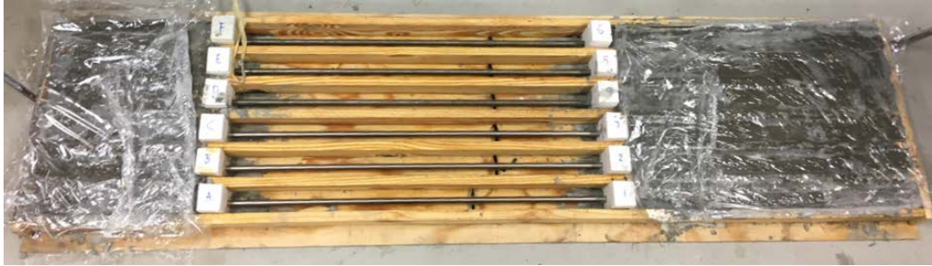
Figure 3.4: Chloride-free concrete batch covered with a plastic film. Polystyrene foam and 3d printed spacers were in place for the chloride-free concrete batch, removed before chloride-contaminated concrete placement.
