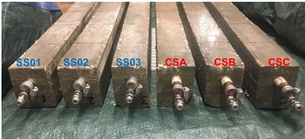
Figure 3.8: Electrical connections at the right end of all specimens. The left end of AISI 1018 CS specimens was epoxy-coated and UNS S41000 SS specimens were not.
