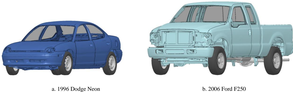
Figure 3.1: Finite element models of two MASH compliant vehicles used in this study.
