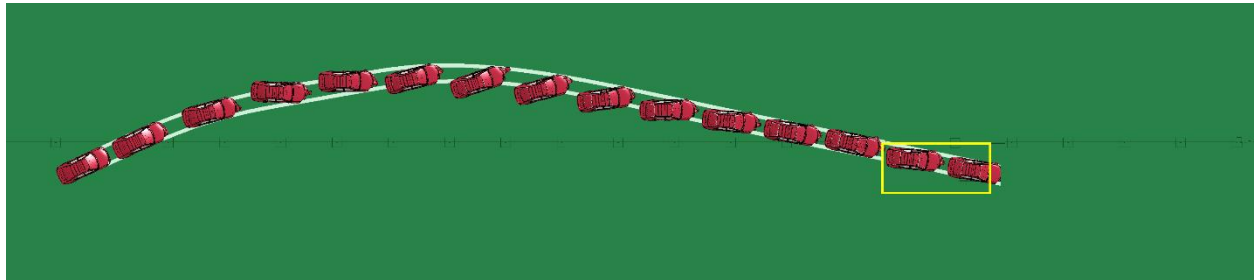
Fig. B.2: A Toyota Camry impacting the current CMB from front-side.
