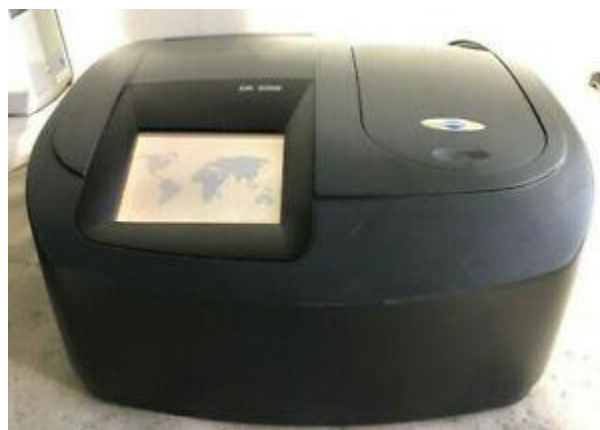
Figure 13. Photo. Hach DR 5000 Spectrophotometer.
