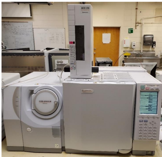
Figure 12. Photo. Shimadzu GCMS-QP2010 SE Gas Chromatograph Mass Spectrometer.
