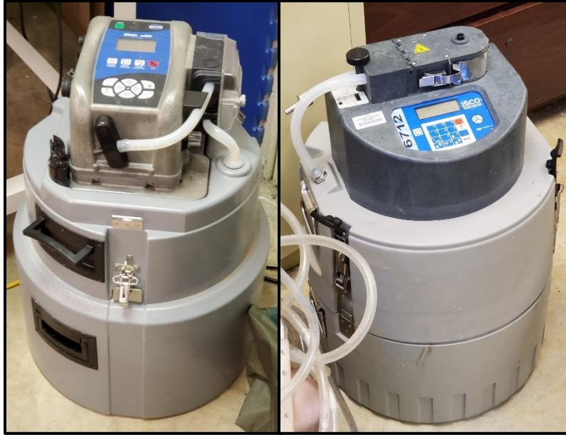
Figure 8. Photos. Hach Sigma SD900 Portable Sampler (left) and Teledyne ISCO 6712 Portable Sampler (right).
