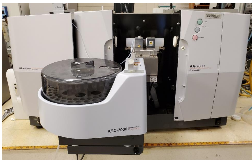
Figure 11. Photo. Shimadzu AA-7000 graphite furnace atomic absorption spectroscopy.
