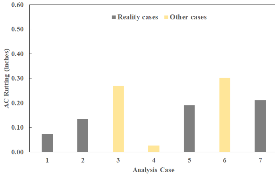
Figure 15. Graph. Impacts of radiation models on asphalt layer rutting prediction in Donalsonville, GA.
