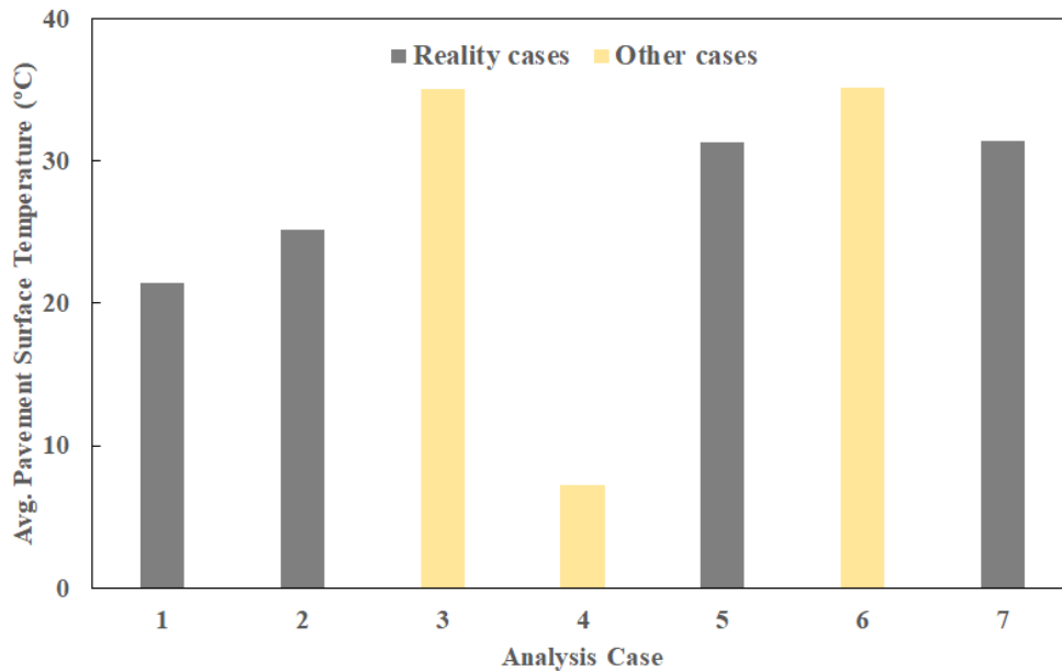
Figure 25. Graph. Impacts of Radiation Models on Pavement Surface Temperature in Donalsonville, GA
