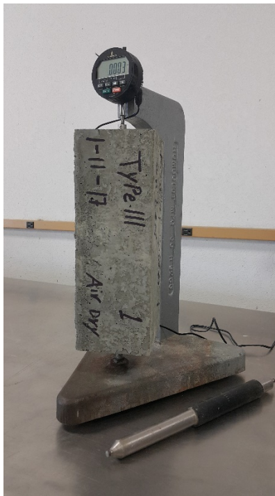
Figure 4-1. Shrinkage strain measurement
