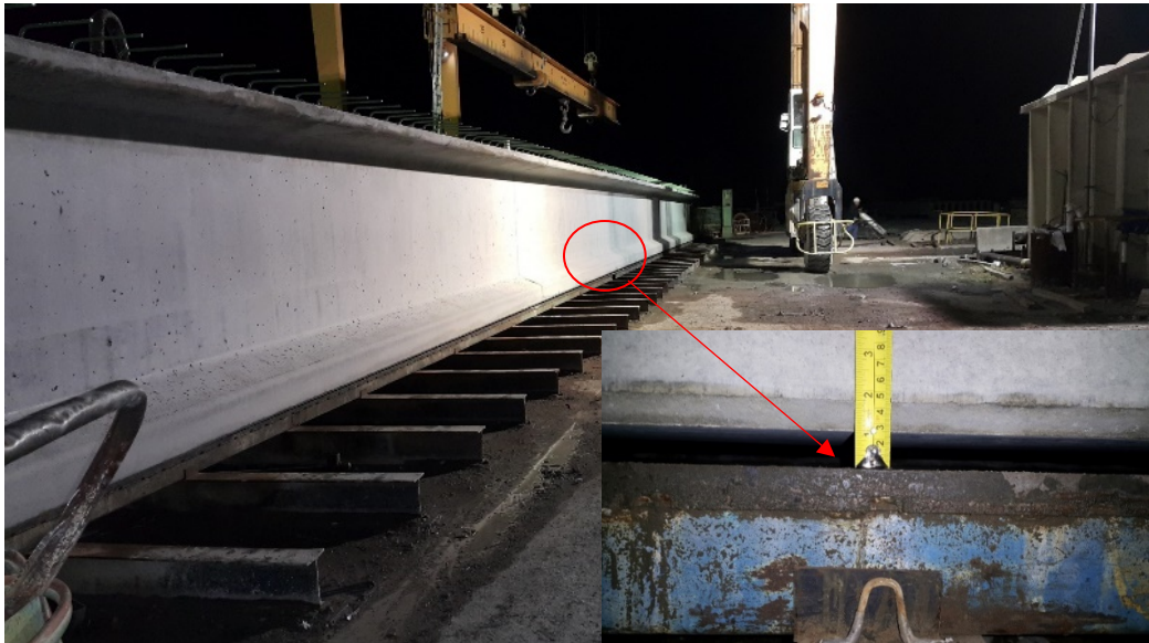
Figure 3-11. Release camber measurement
