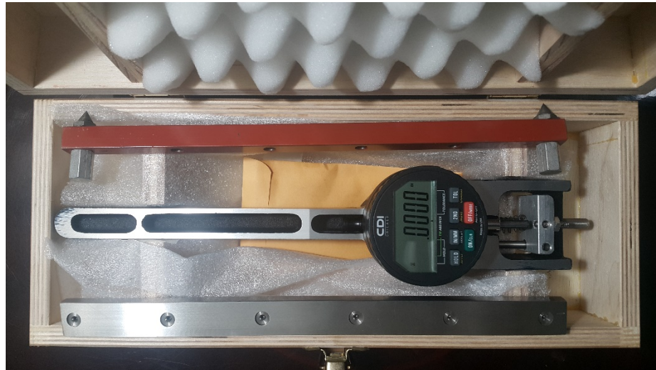
Figure 4-4. DEMEC gage device used in creep strain measurements
