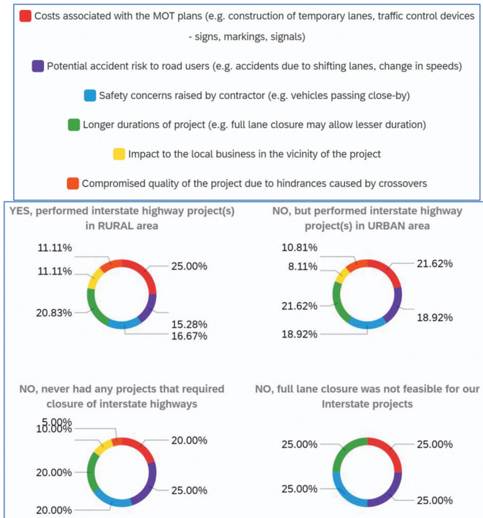
Figure 4.5 Advantages of full/one direction closure over crossovers.
