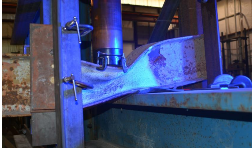
Figure 8. Example of Beam Lifting at End Because of Applied Loads
