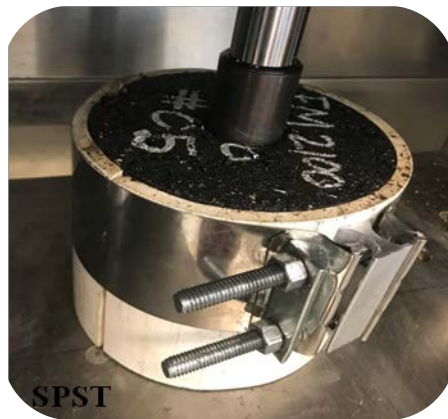
Figure 4. SPST specimen setup.
