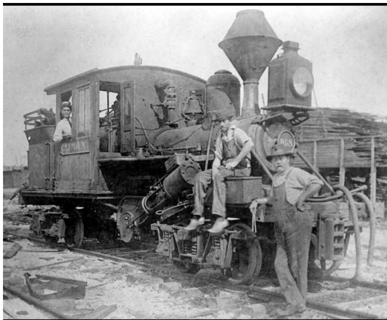
A Climax engine, used by logging railroads in Georgia mountains (S. Storey)
