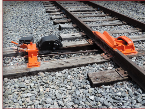
Derail device, Elko (Houston County)
