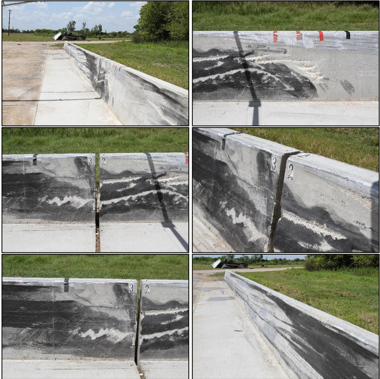
Figure 6.3. TxDOT Shallow Anchorage SSTR without Dowel Bars after Test No. 469680-02-2.
