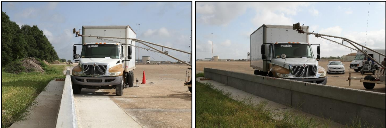
Figure 6.1. TxDOT Shallow Anchorage SSTR without Dowel Bars/Test Vehicle Geometrics for Test No. 469680-02-2.
