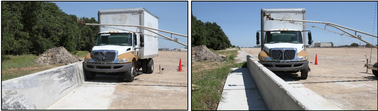
Figure 7.2. TxDOT Shallow Anchorage SSSTR without Dowel Bars and with Concrete Apron Extended Downstream of Barrier/Test Vehicle Geometrics for Test No. 469680-02-3.
