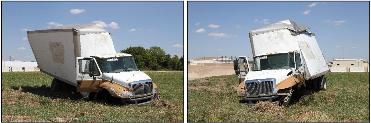
Figure 7.7. Test Vehicle (Uprighted) after Test No. 469680-02-3.
