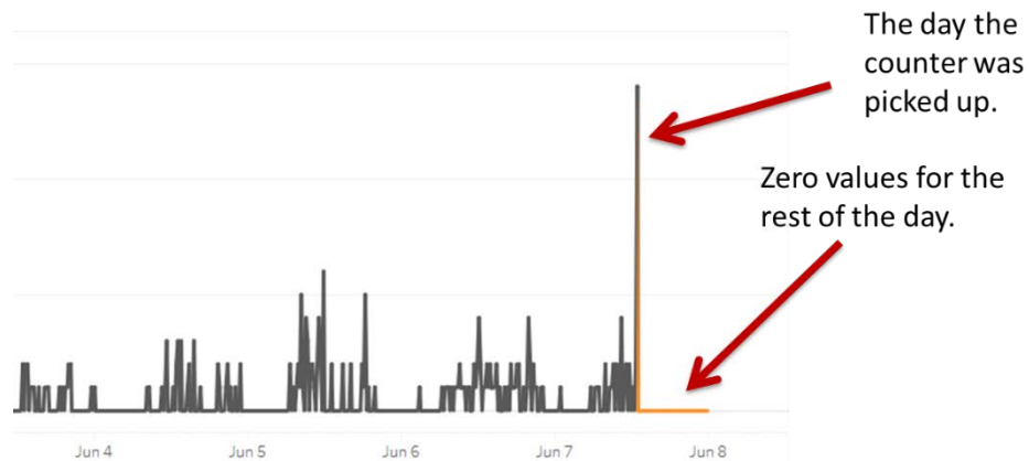
Figure 11. Bad Data Example: Partial Day Count with Spike When Counter Retrieved.
