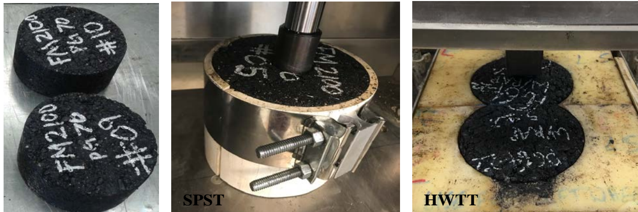
Figure 3. Typical HMA Samples for the SPST and HWTT Tests.
