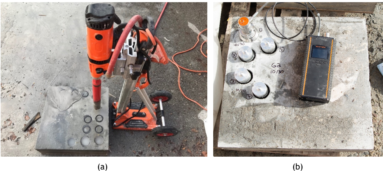
Figure 6. Pull-off testing procedures: (a) coring and (b) testing
