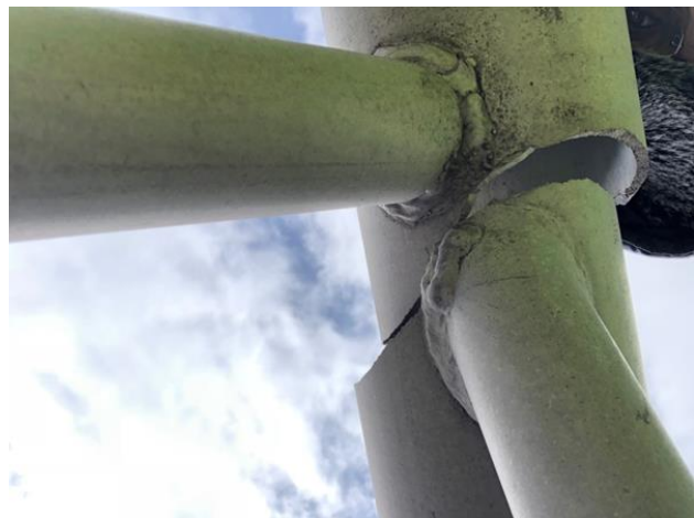
Figure 2: Complete fracture observed at one location within the truss
