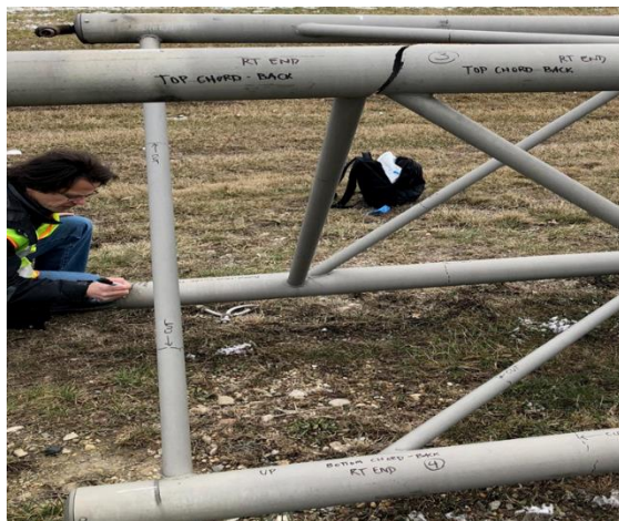
Figure 2: Complete fracture observed at one location within the truss
