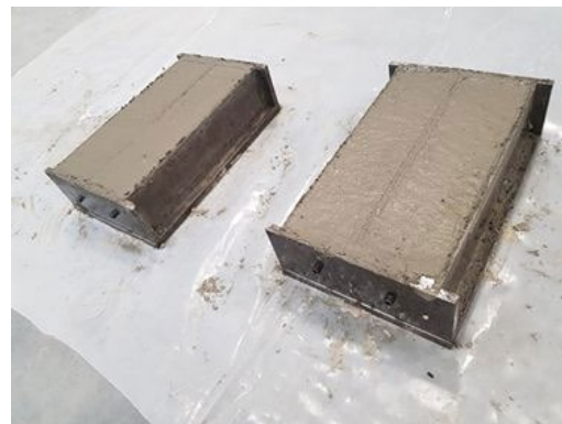
Figure 4.1 CPT molds a) without prisms and b) with prisms
