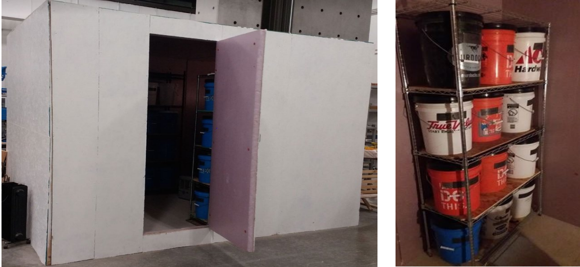
Figure 4.5 CPT prism storage oven a) outside and b) inside
