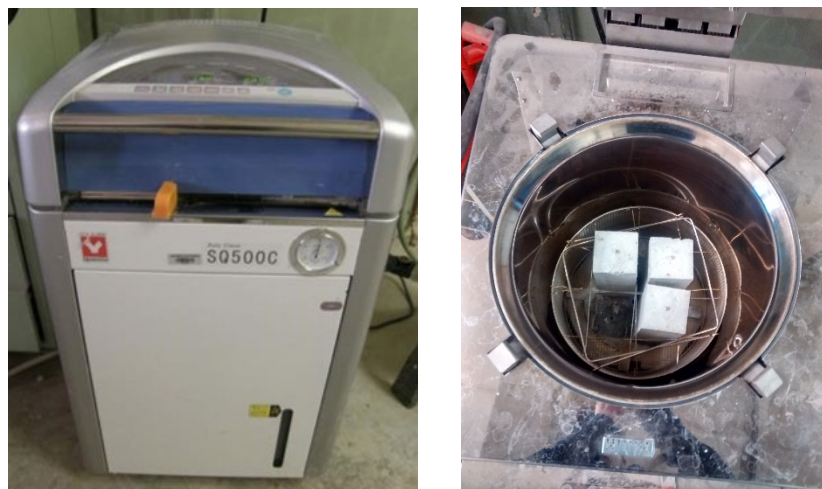
Figure 4.7 Autoclave a) exterior and b) interior with prism
