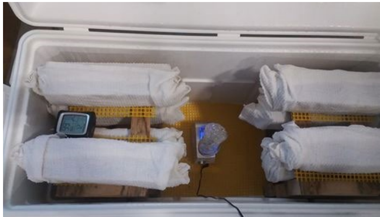
Figure 4.6 CPT prisms in alternative curing chamber
