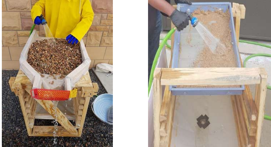
Figure 3.5 Washing process a) coarse aggregates and b) fine aggregates
