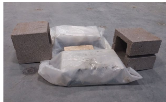
b) Molds wrapped with plastic sheet
