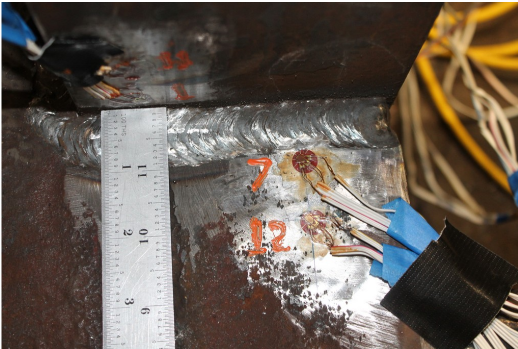
Figure A-8. Strain Gauges 7 and 12
