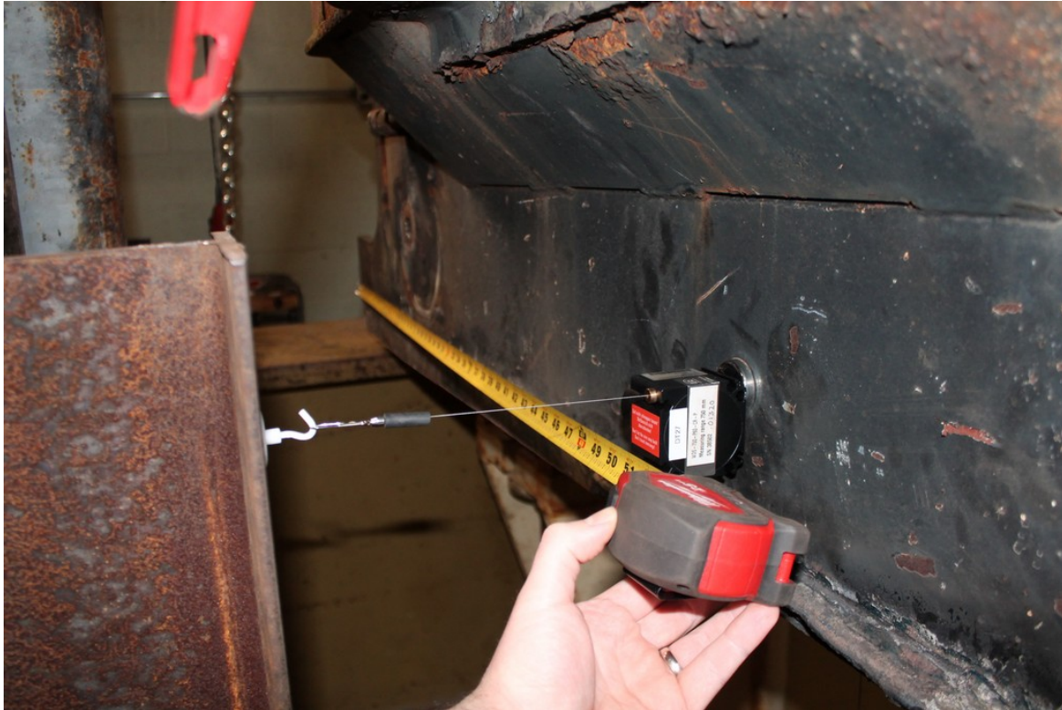
Figure 12. Longitudinal String Potentiometer on the Underframe
