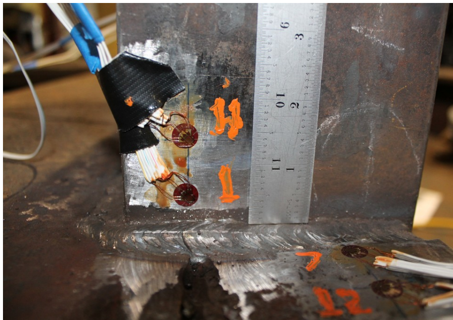
Figure A-2. Strain Gauges 1 and 11
