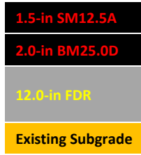
Figure A.9. Structure for the SR10 FDR Project (Chesterfield County)
