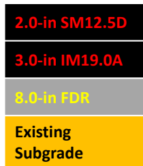
Figure A.13. Structure for the SR620 FDR Project (York County)
