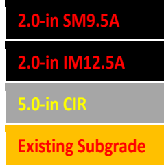
Figure A.22. Structure for the SR60 CIR Project (Henrico County)
