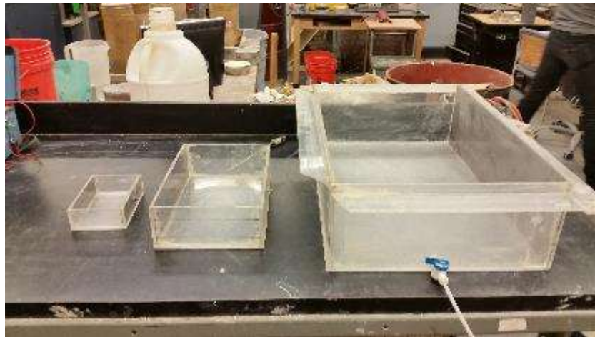
Figure 2.3-Original, Doubled Dimension and Quadrupled Dimension Two-Electrode Resistivity boxes
