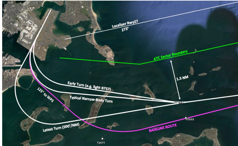
Figure 28. Procedure illustration for a 22R departure climbing via the BLZZR4 departure (baseline) compared to procedure 1-D3b.
