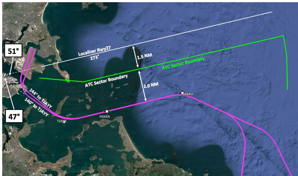
Figure 26. Current RNAV SIDs from Runway 22L and 22R (magenta), ILS Localizer to Runway 27 (white) and the air traffic control sector boundary (green).
