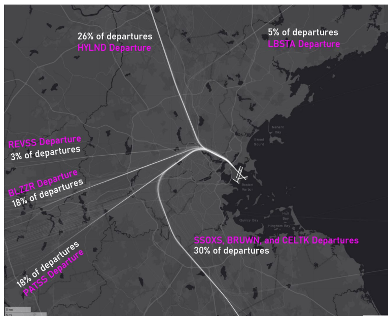
Figure 34. Current RNAV departure procedures from Runway 33L.
