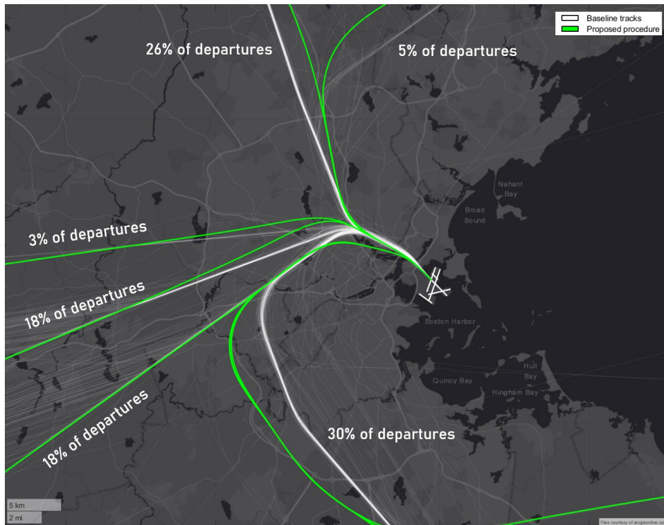
Figure 42. Baseline radar tracks from 2017 (white) are compared to simulated flight tracks of aircraft flying the proposed procedure (green).
