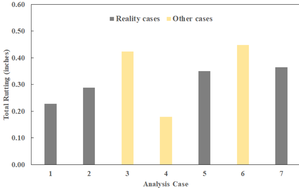
Figure 11. Graph. Impacts of radiation models on total rutting prediction in Jeffersonville, GA.
