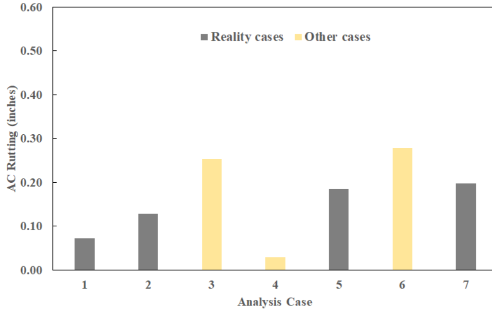
Figure 16. Graph. Impacts of radiation models on asphalt layer rutting prediction in Jeffersonville, GA.
