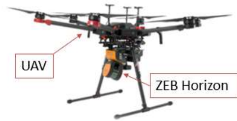
UAV SLAM ZEB Horizon with quick release UAV mount LiDAR point clouds in minutes
