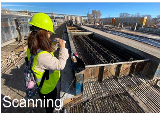
Figure 31. Field Testing using Azure Kinect scanner in CoreSLAB.
