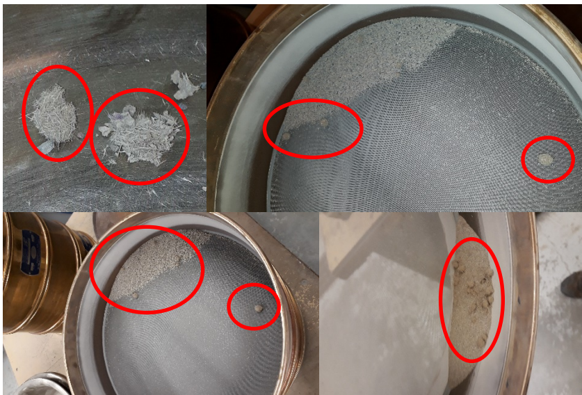
Figure A-1. Fibers Existing with the Aggregate after the Extraction Process of Asphalt Binders from Mixes Containing RAS
