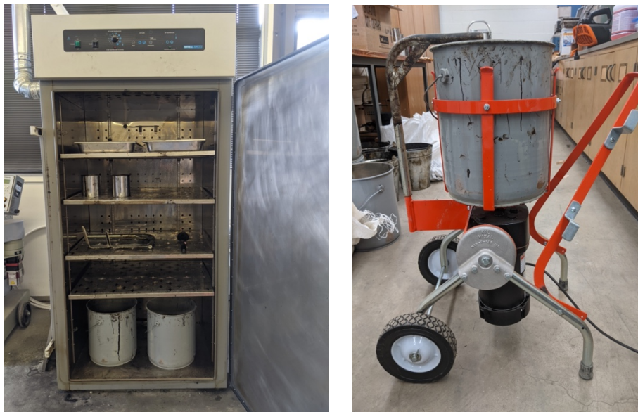
Figure 1. (a) Aggregate, Binder, Mixing Bucket, Spatula, and Mixing Paddle Conditioned at Force Draft Ovens; (b) Mobile Bucket Mixer with Mixing Bucket
