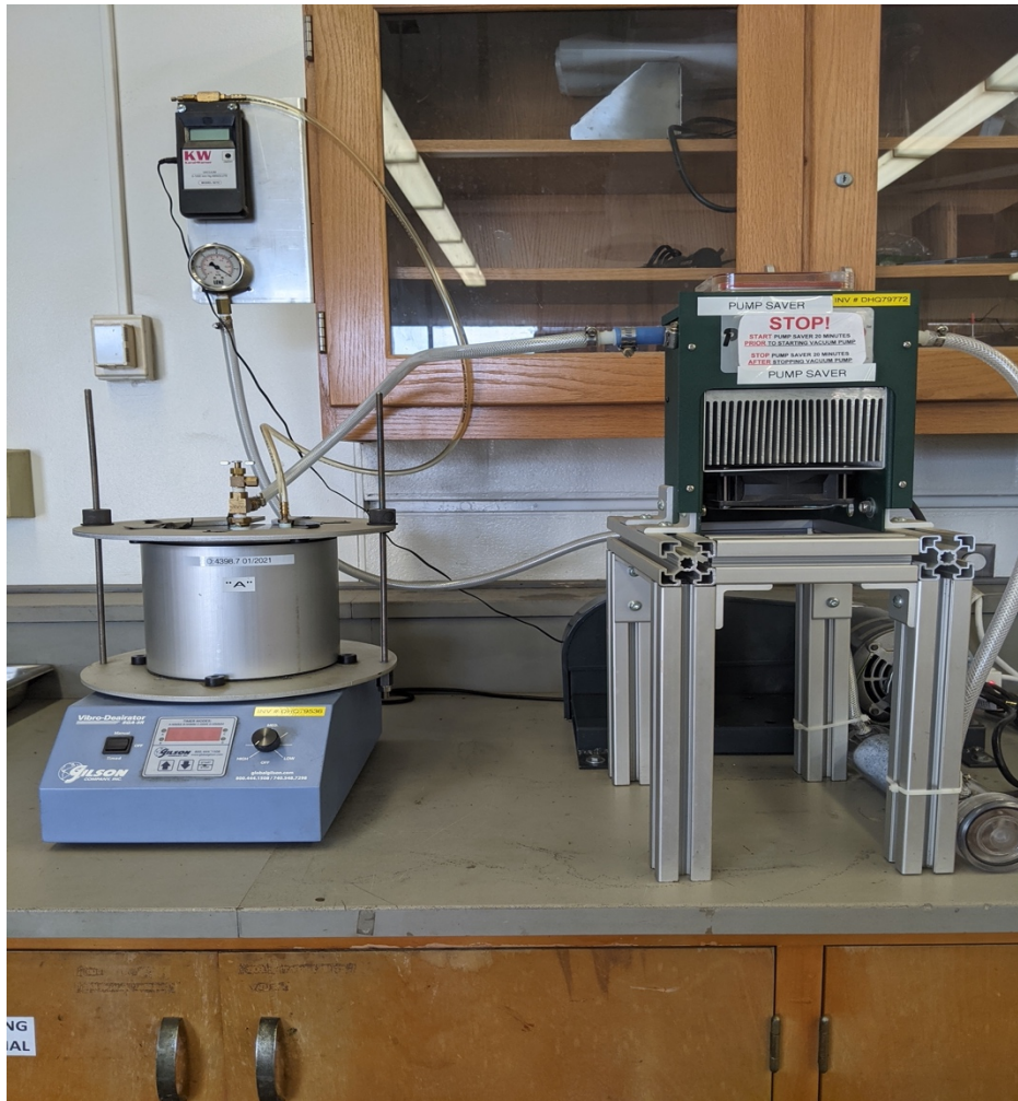
Figure 3. Apparatus Setup Consisting of Pycnometer, Vacuum Pump, and Mechanical Shaker for Determining G_{mm}
