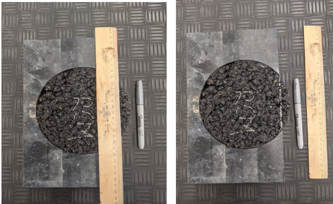
Figure 5. Marking of Cut Line for Hamburg Wheel Tracking Test
