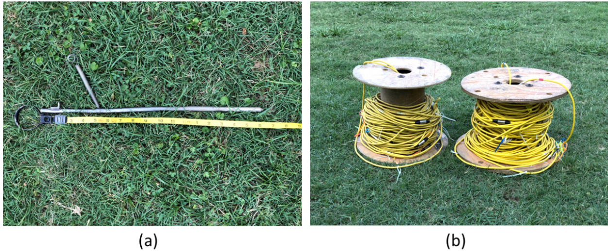
Figure 3.9 (a) a stainless-steel electrode and (b) multi-electrode cable sections each includes 14 take-outs
