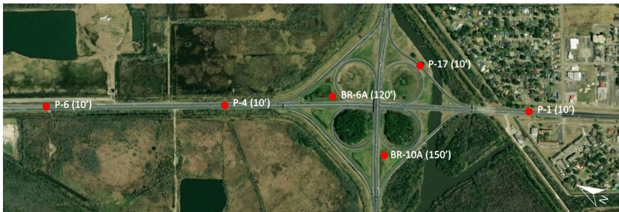
Figure 4.5 Locations of the boreholes along with the depth of borings in Beaumont district
