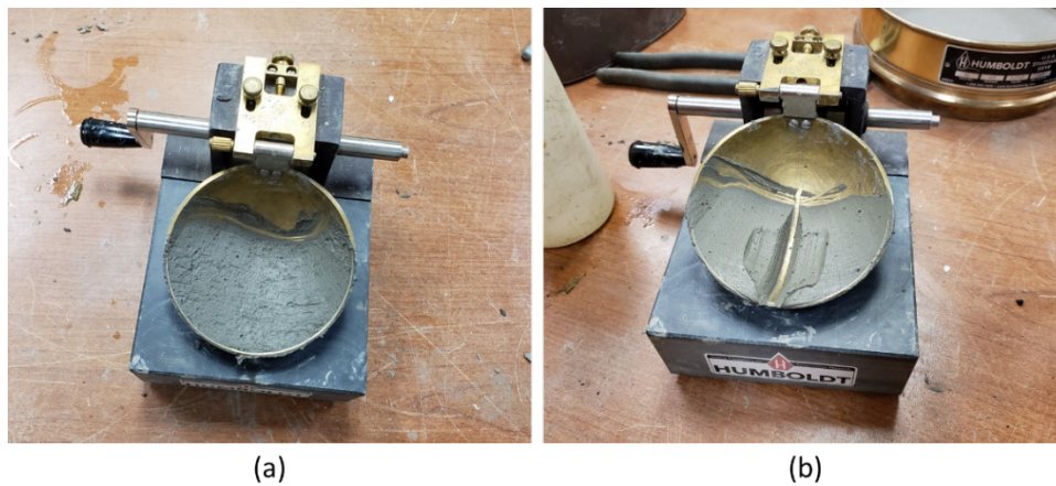
Figure 4.13 Liquid limit testing: (a) the soil is flattened in the device cup, and (b) a groove was made at the center (UTA laboratory)
