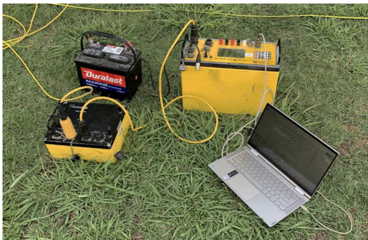
Figure 3.23 Proper connection of resistivity meter to an external battery, a switching system, and a laptop
