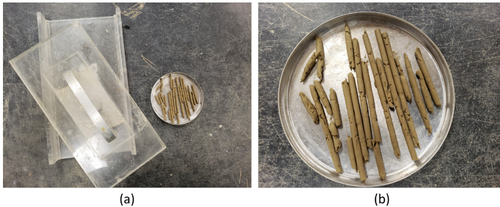
Figure 4.14 Plastic limit testing (a) Rolling device and (b) cracked and broken threads of 3 mm (UTA laboratory)
