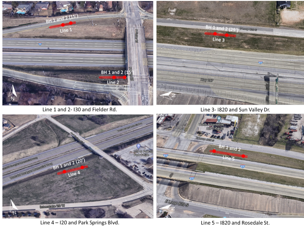
Figure 4.11 Locations of resistivity lines with respect to the boreholes along with the depth of borings in Fort Worth district
