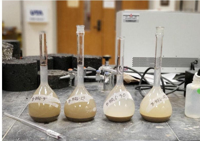
Figure 4.16 Specific gravity testing of soil (UTA laboratory)
