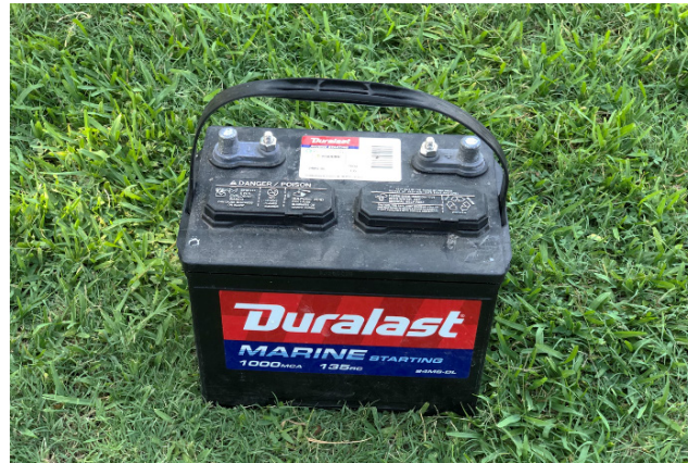
Figure 3.11 External marine 12 V battery
