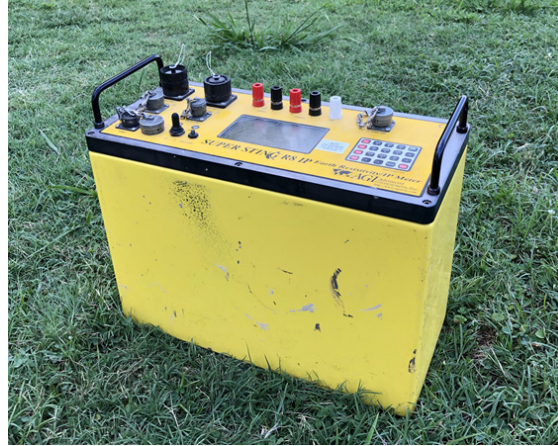
Figure 3.7 AGI Supersting R8 resistivity meter
