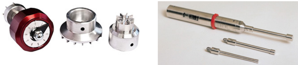
Figure 2.4 Torvane device (left); Pocket penetrometer with different sizes of the adaptor (right)
