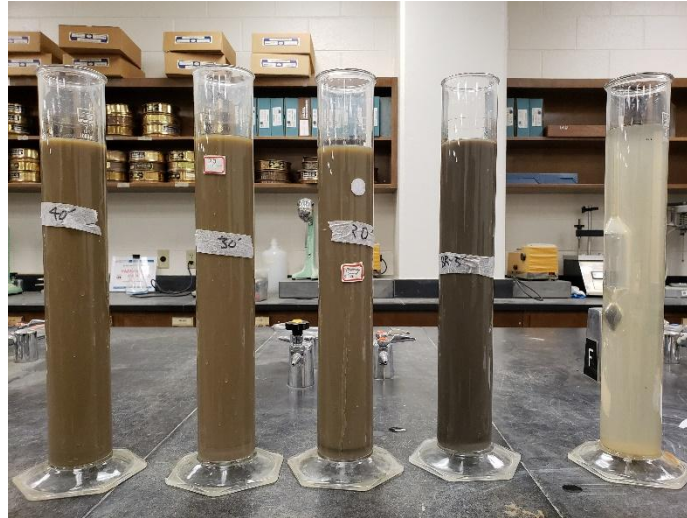
Figure 4.15 Particle size distribution testing using the hydrometer procedure (UTA laboratory)
