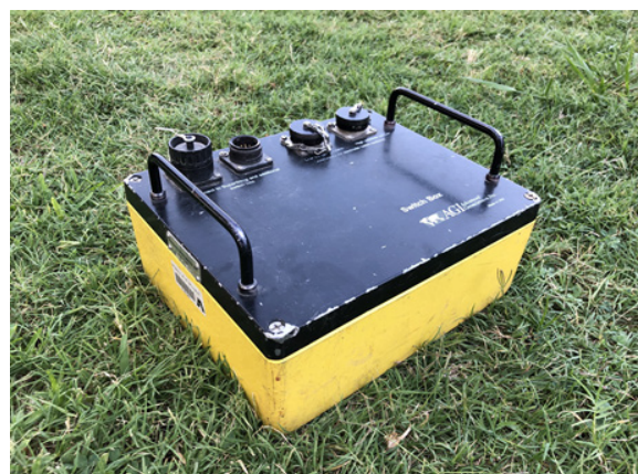
Figure 3.12 AGI switch box
