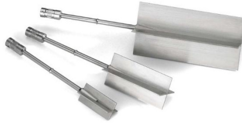
Figure 2.3 Examples of different sizes of vane shear blades (johnmorriscgroup.com)
