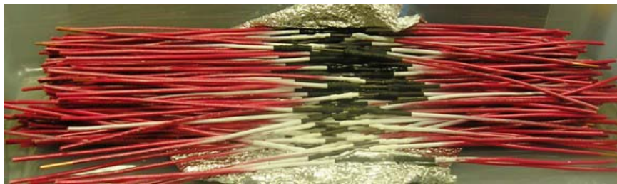
Figure 5. Custom-made chloride sensors (dark color) welded to copper wires (red color), before being embedded in the concrete samples.
