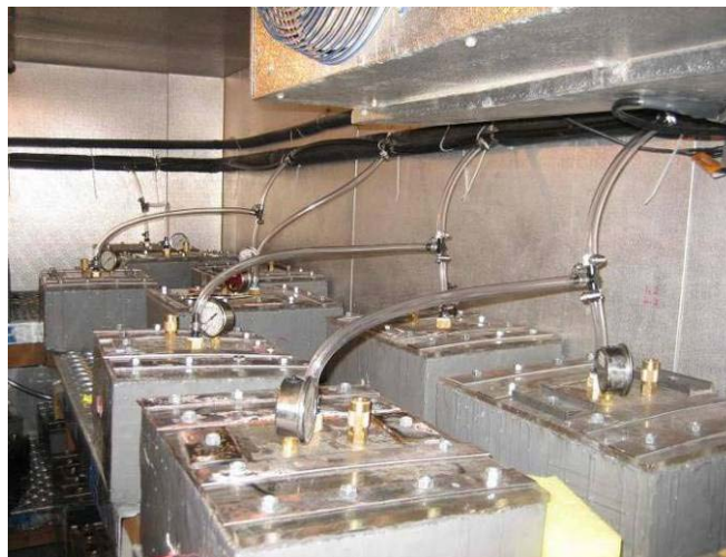
Figure 8. (a) Schematics and (b) experimental setup for the pressurized transport of deicers into concrete
