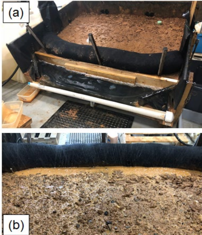
Figure 11. Images from the simulated events using the straw sediment tube. (a) The installed tube shows the posts were ~0.61 m (2.5 ft.) apart. (b) Sediment-laden runoff begins to pond behind the silt fence.
