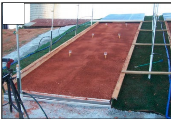
Figure 2. The standard method TM11340. (a) Example of the large-scale test structure used under the method. This is a bare soil test to provide baseline erosion rates. (b) Typical results from the TM11340 tests. It is a plot of soil loss vs. the R-factor of the USLE equation. From Sprague and Sprague (2012).
