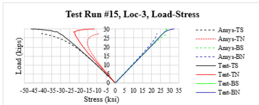
Figure 92. Comparison of Loc. 3 stresses between analysis and test data, Test Run #15
