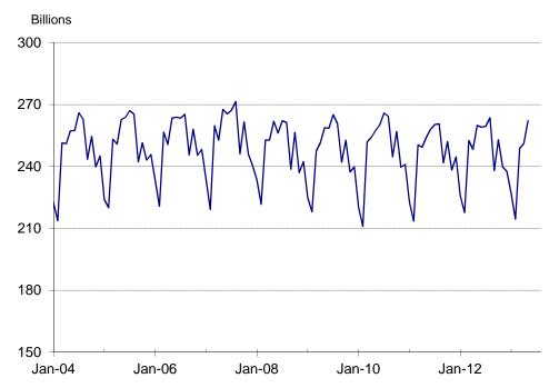
Vehicle-miles traveled (VMT) are key data for highway planning and management, and a common measure of roadway use. Along with other data, VMT are often used in estimating congestion, air quality, and potential gas-tax revenues, and can provide a general measure of the level of the nation's economic activity.
