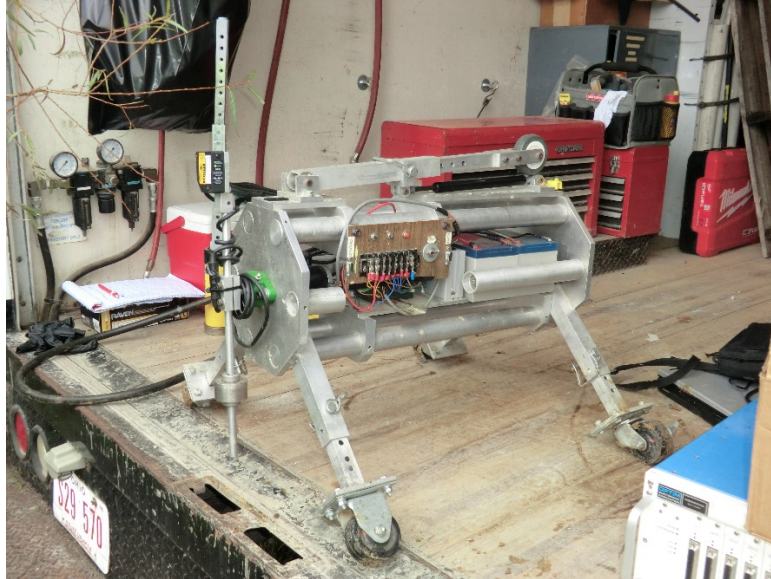
Figure 1. Direct Measurement Mandrel developed in 2002 by Ohio University [Sargand et al., 2002].
