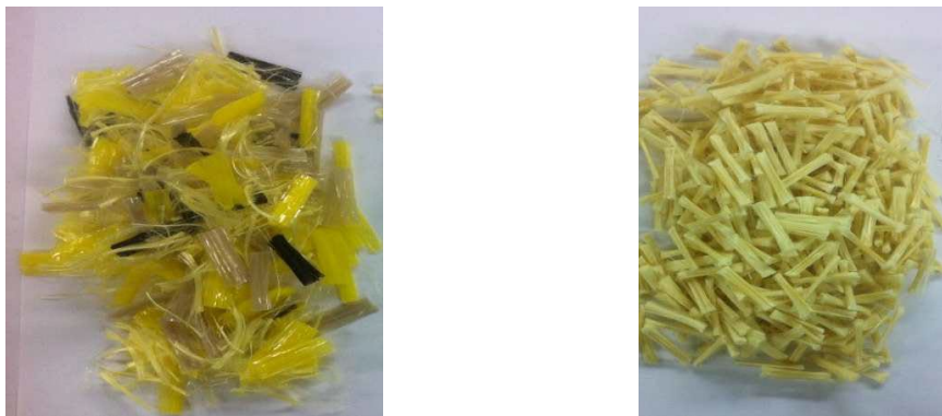
Figure A.1. Main Types of Aramid Fibers: a) Blend of Aramid and Polyolefin Fibers, b) Wax-Treated Aramid Fibers.
