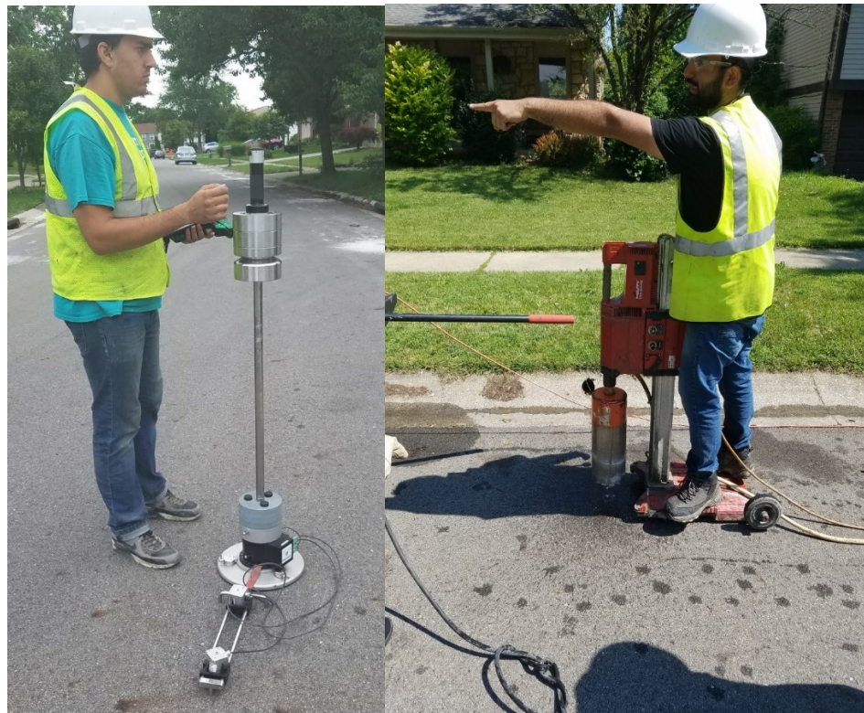
Figure B.2. Light weight deflectometer (LWD) measurement (left) and coring (right) at the field.
