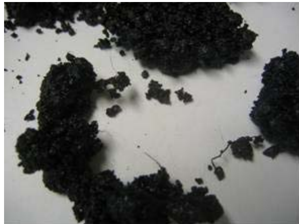
Figure A.2. Loose Sample of a Plant-Produced Fiber-Reinforced Asphalt Mixture (7)
