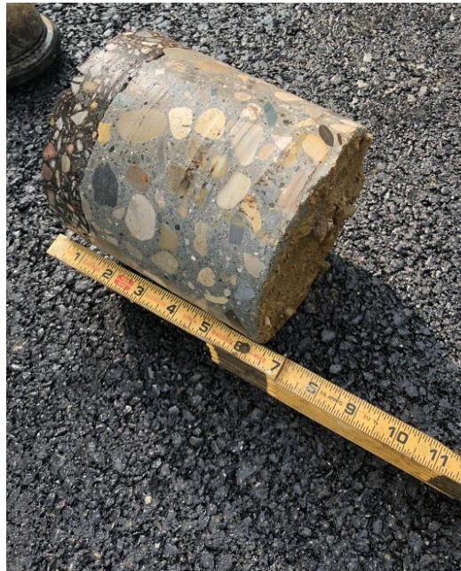
Figure A.12 Picture of Core Obtained from the City of Columbus Project with an Overlay Placed on Concrete Pavement
