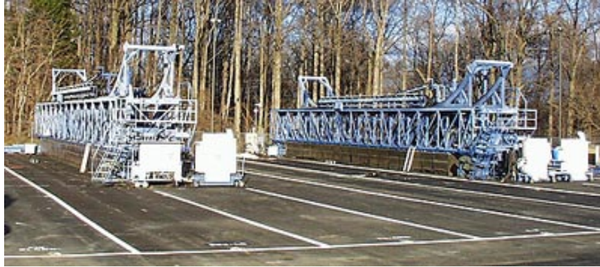
Figure E.1 FHWA Pavement Test Facility (PTF) shown with two Accelerated Loading Facility (ALF) machines
