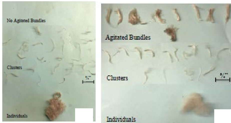
Figure A.4. Aramid Fibers Extraction State from a Single Sample; a- Blend of Polyolefin and Aramid Fibers, b- Wax-Coated aramid (15)
