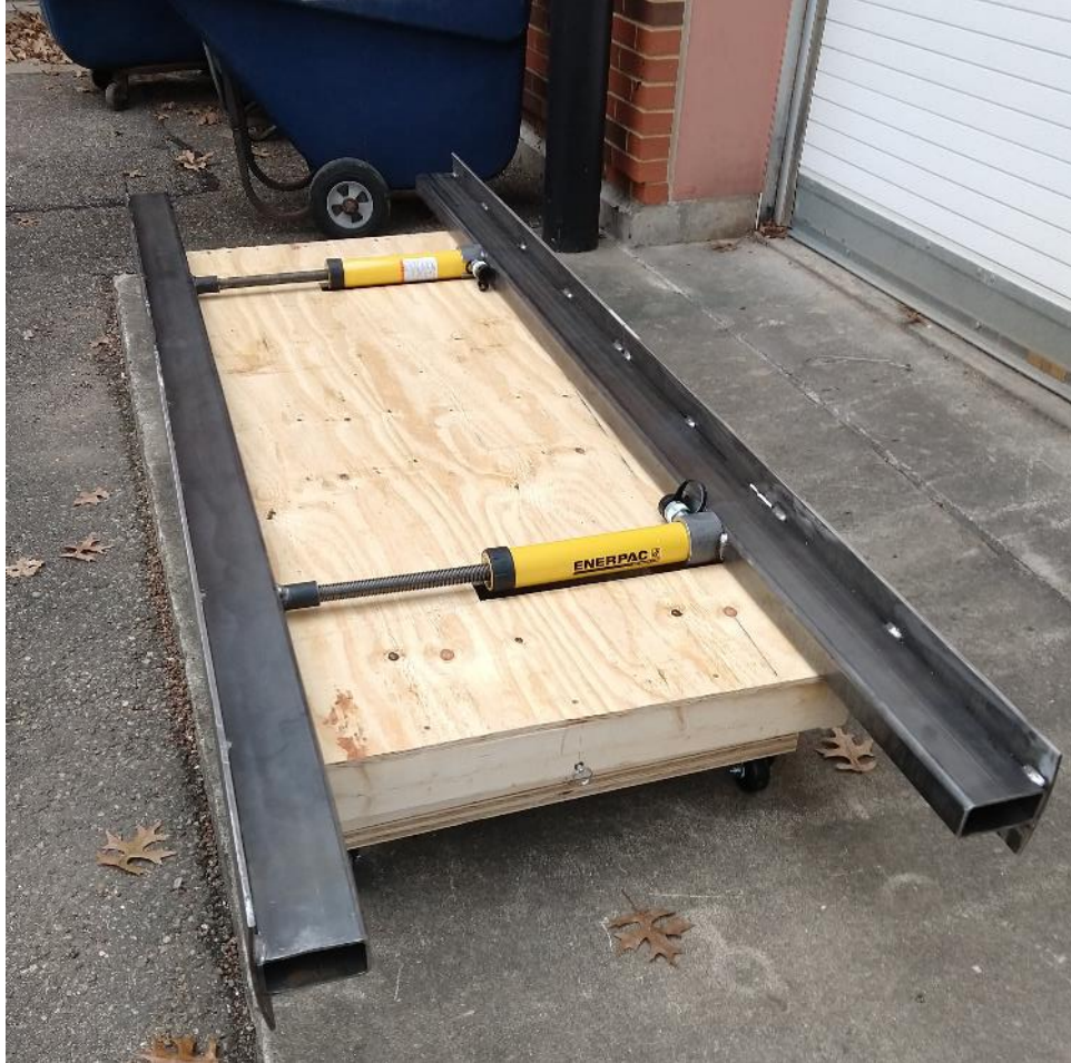
Figure 40. Pipe deflector assembled at ORITE laboratory.
