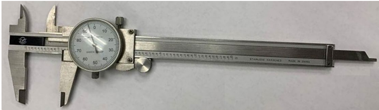
Figure 21. Calipers used to measure corrugation depth. The right end was extended into a hole until it touched the crest of the corrugation.
