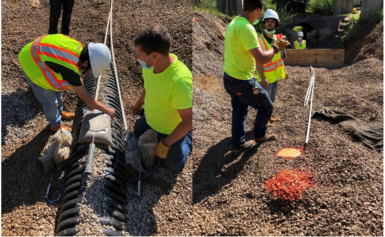
Figure 48. Installation of sensors around Test Pipe 4. Left: Pressure cell placed over crown. Right: Accelerometers and colored aggregate.
