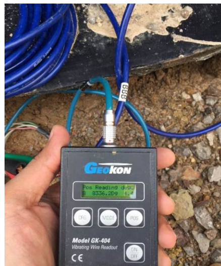
Figure 25. Geokon vibrating wire readout device.
