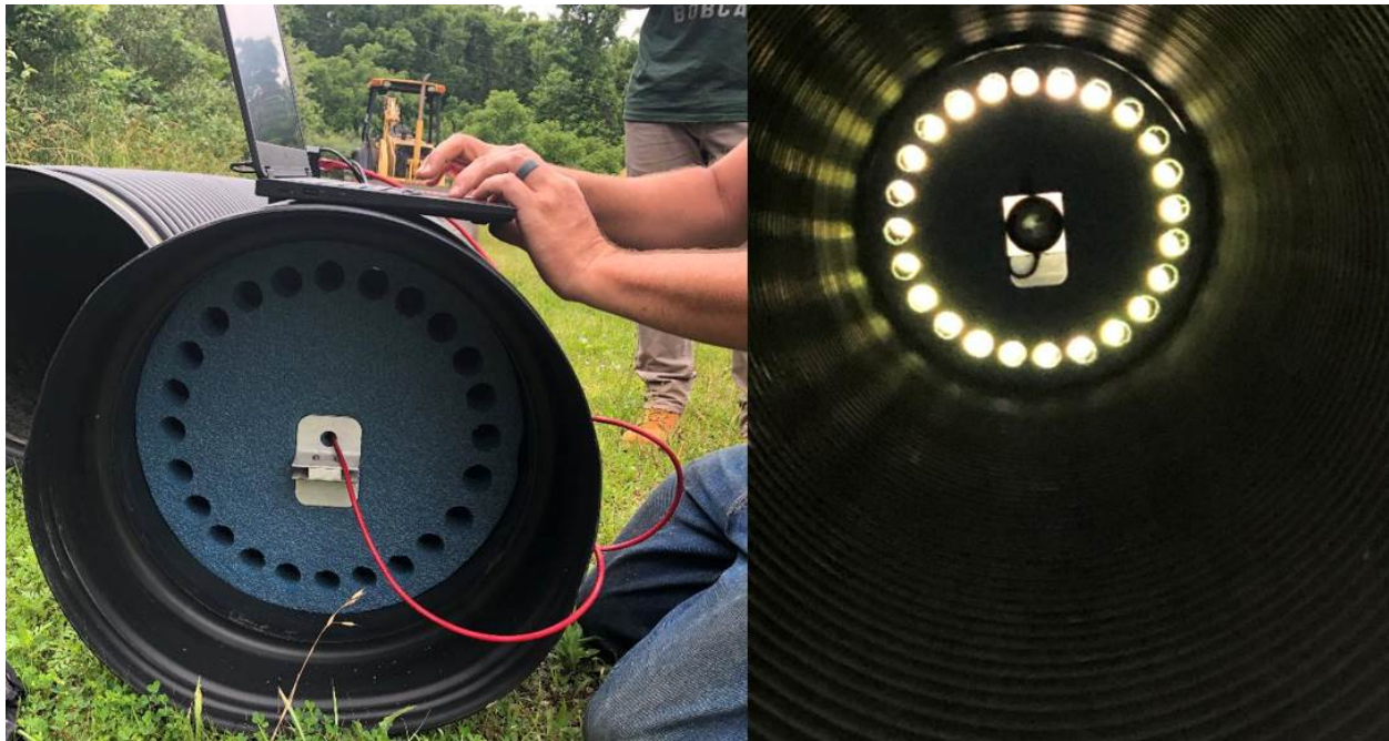
Figure 46. LiDAR pipe profiler in use. Left: Profiler placed in pipe and connected to controller laptop. Right: View of profiler from inside pipe.
