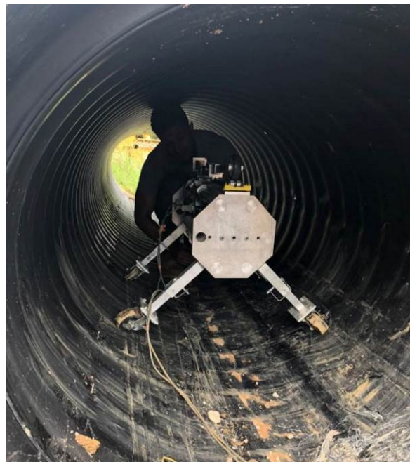
Figure 19. Laser profiler recording a cross-sectional profile.
