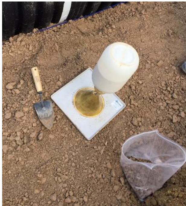
Figure 26. Sand cone test.
