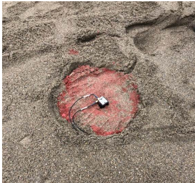
Figure 32. Upper accelerometer 18 in (460 mm) above pipe crown with red sand surrounding.
