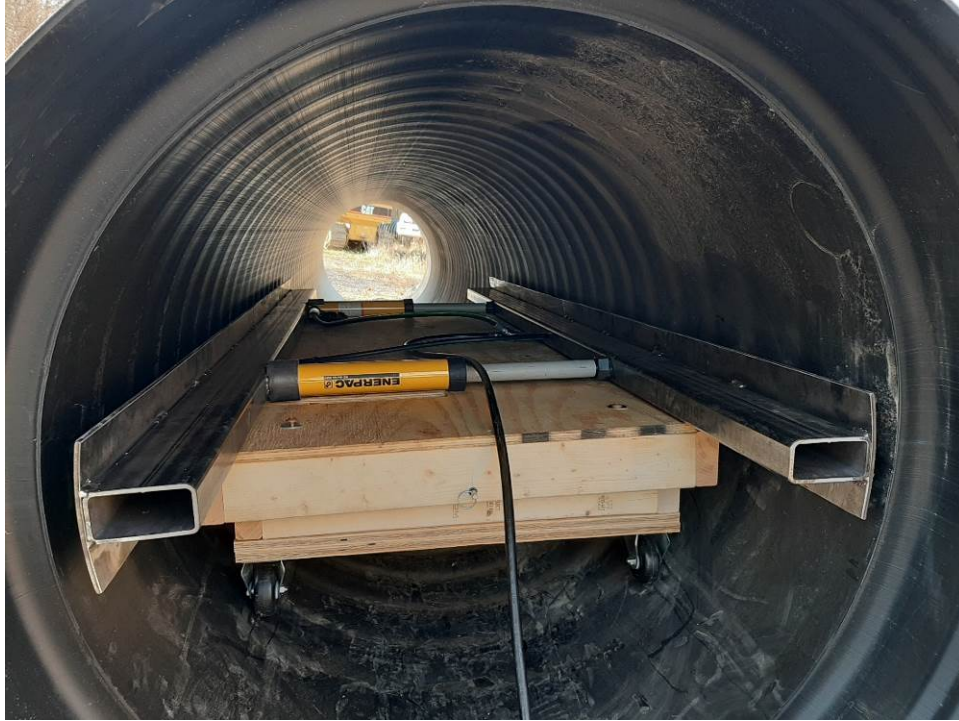
Figure 42. Actuated deflection device and delivery system deforming Pipe 3.
