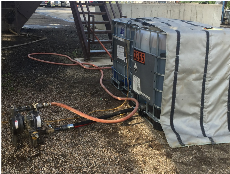
Figure B.3: Introduction of Aromatic Oil into the Asphalt Binder Line at the Asphalt Plant in Medina County.
