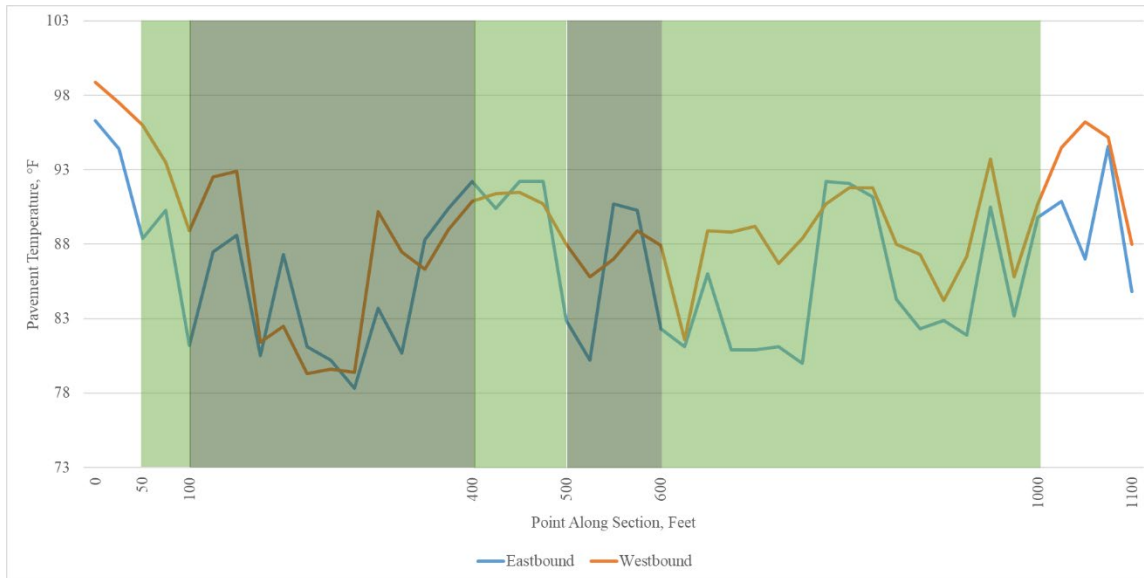
Surface temperature levels measured by FLIR – SR 676 (2) in Washington County, Ohio
