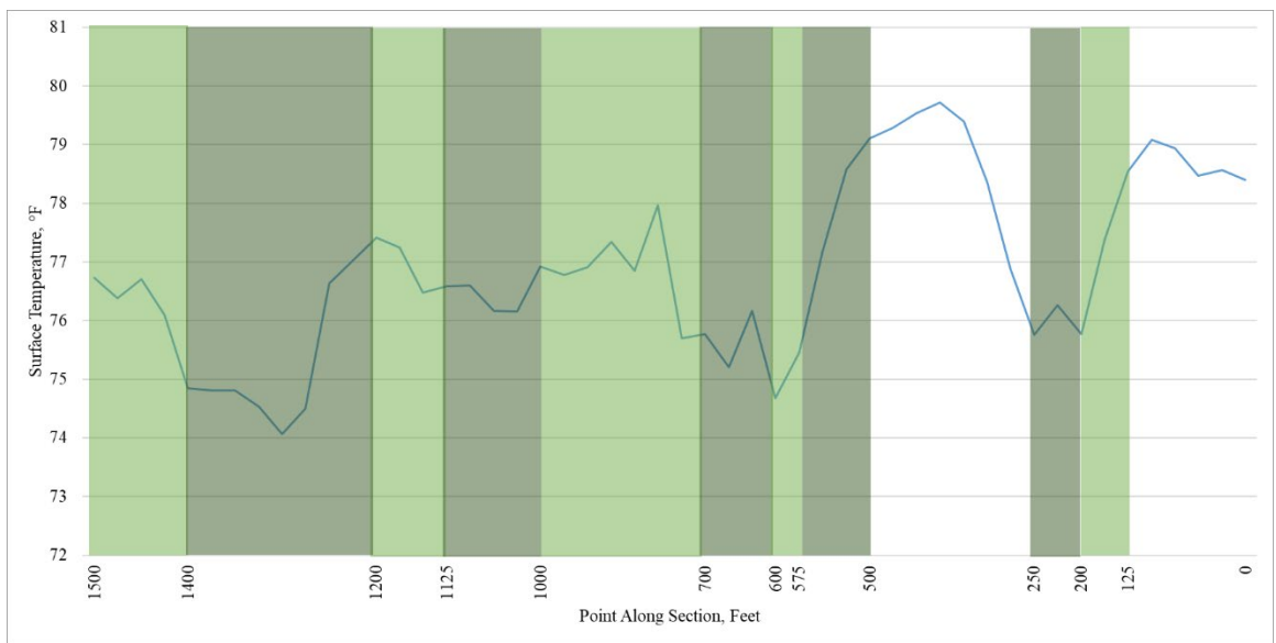
Surface temperature levels measured by MARWIS – SR 800 (1) (SB) in Tuscarawas County, Ohio
