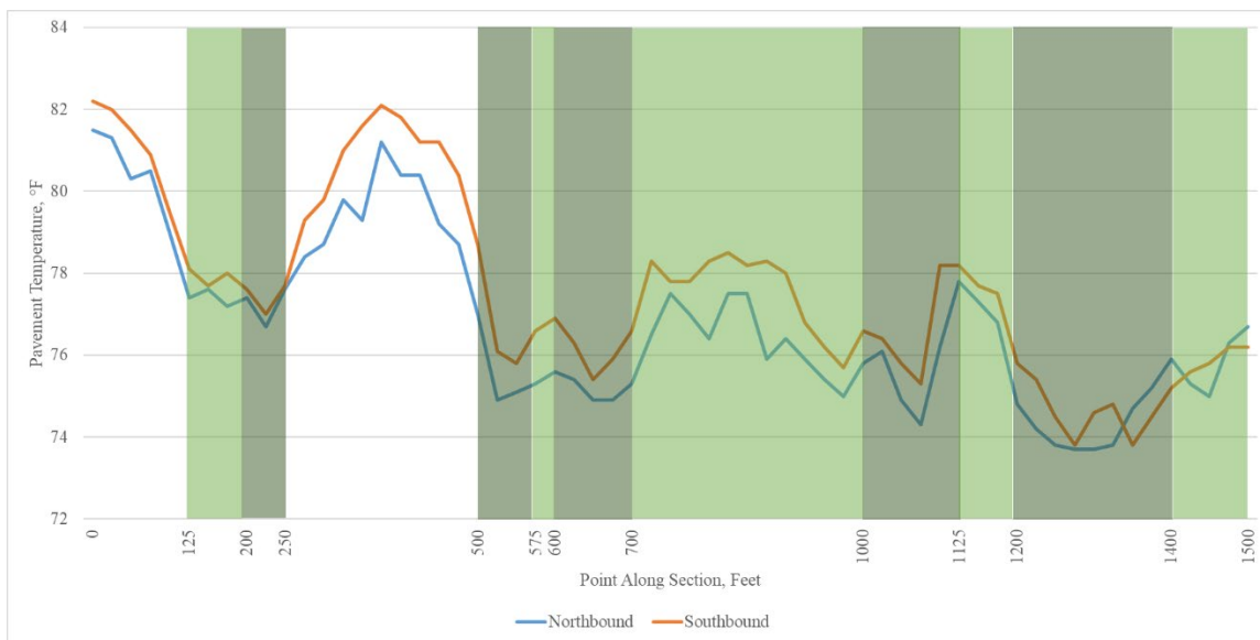
Surface temperature levels measured by FLIR – SR 800 in Tuscarawas County
