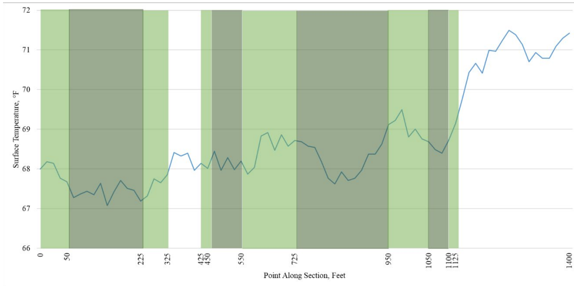
Surface temperature levels measured by MARWIS – SR 139 (EB) in Scioto County, Ohio
