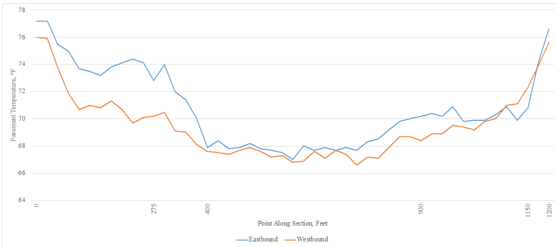
Figure C12. Measured Temperature Levels on SR 124 (2) (EB, WB) in Jackson County, Ohio (1 ft = 0.305 m, Temperature range 17.8°C to 25.6°C)
