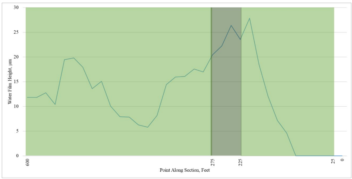
Measured moisture level - SR 327 (1) (SB) in Vinton County, Ohio
