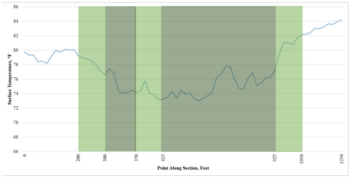
Surface temperature levels measured by MARWIS – SR 56 (WB) in Hocking County, Ohio
