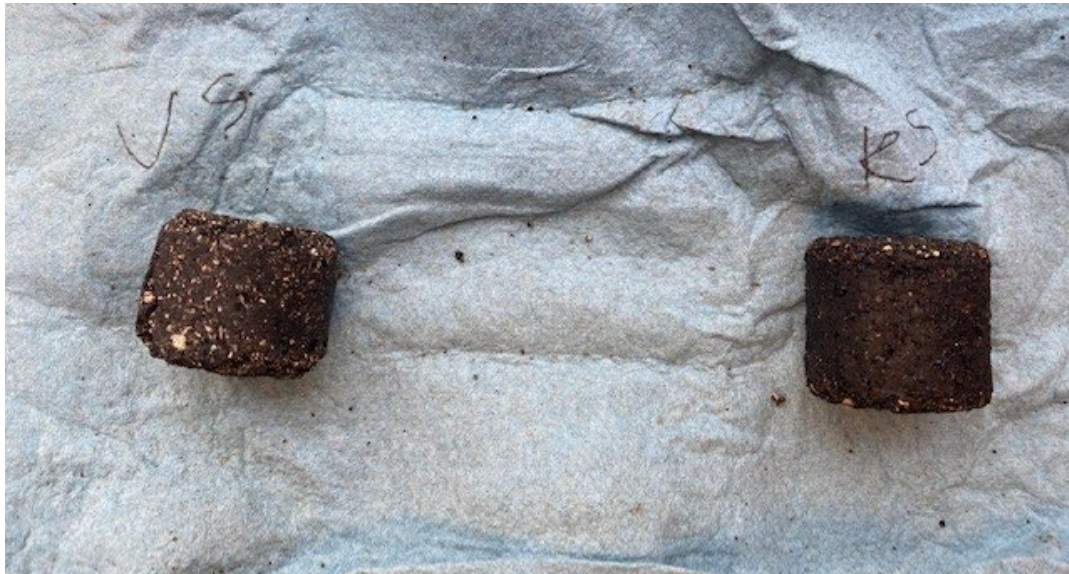
Figure 9-6 Pills at the Conclusion of ISSA TB 144 Testing; Virgin Aggregate on the Left and RAP on the Right
