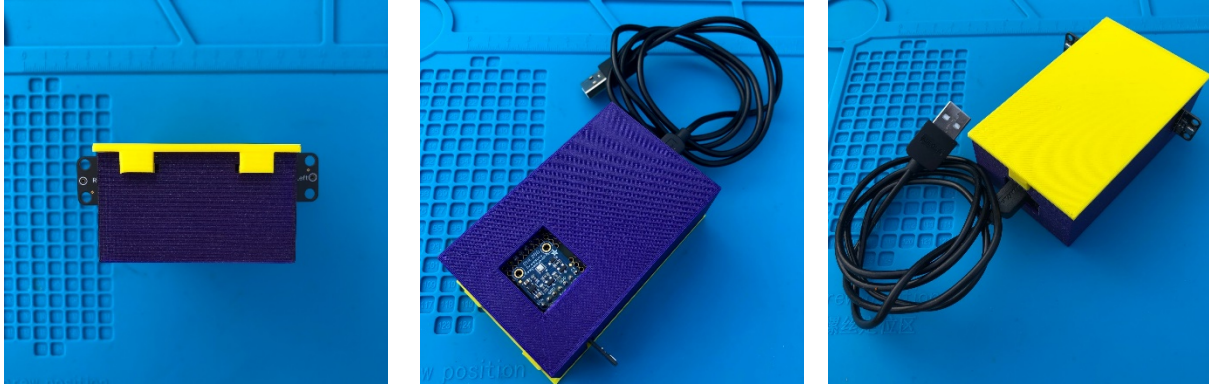
Figure 7. Pictures of the developed prototype device with 3D-printed housing. The size is 88 x 55 x 30 mm 3 .
