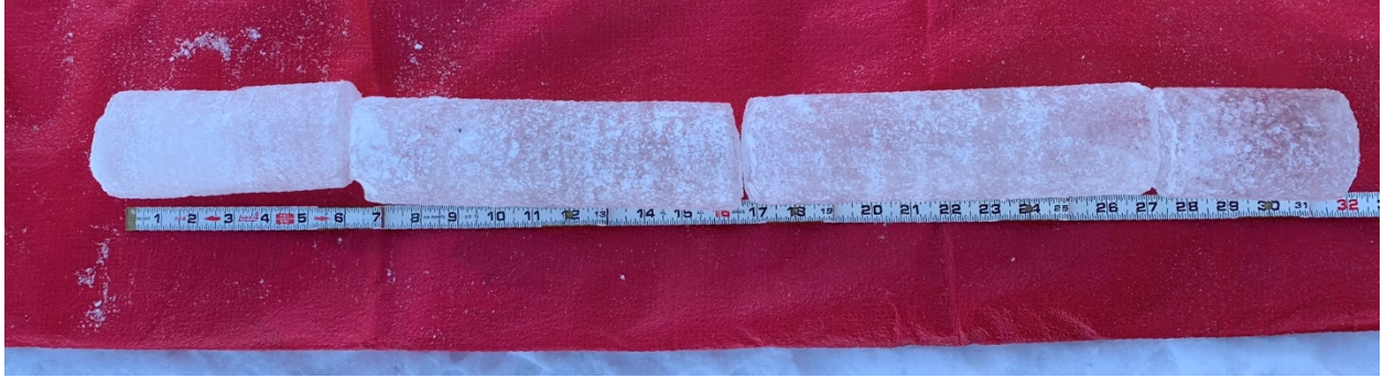
Figure 4.8 Photograph of a 0.80-m-long ice core collected from the trench road.
