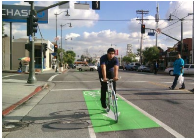
Figure 2.1. Green conflict paint used to enhance bike lane visibility (NACTO, 2012).
