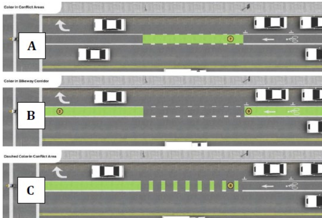
Figure 2.2. Three design alternatives for conflict zones at right turn pockets (NACTO, 2012).
