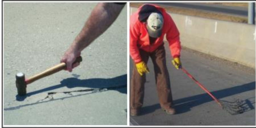
Figure 67. Photo. Sounding deteriorated concrete using a hammer (left) and steel chain (right) (Frentress et al., 2012)
