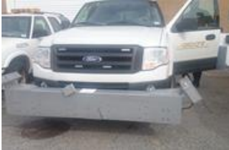
Figure 179. Photo. Laser Profiler for IRI Collection
