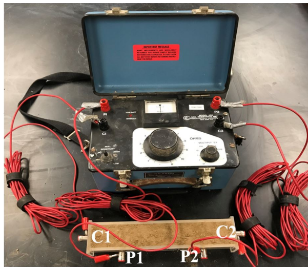
Figure 3.4: Soil box for laboratory resistivity measurements
