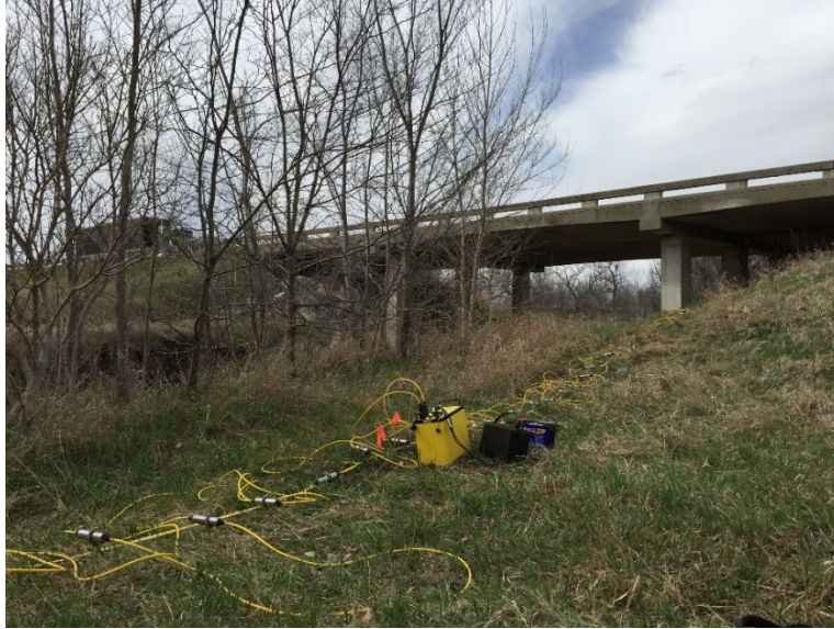
Figure 3.3: Field ERT data acquisition system, flags indicate where boreholes will be located
