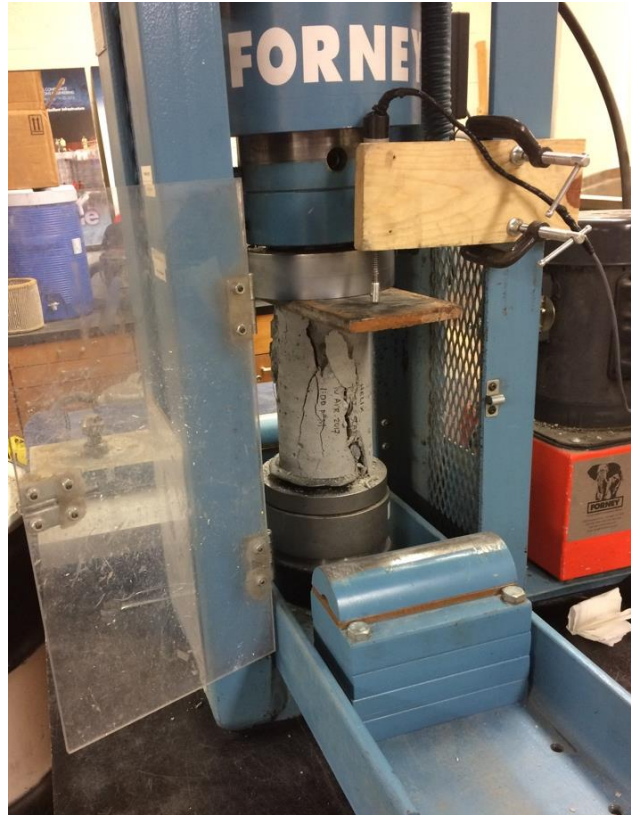
Figure 3-9 Compressive strength testing.
