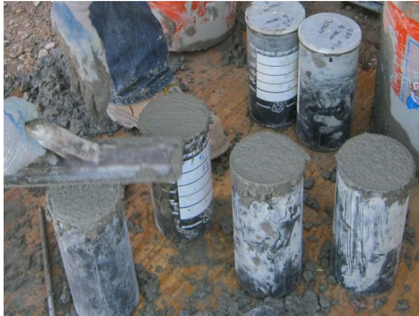
Figure 3-5 Casting of cylindrical specimens during construction of bridge decks.
