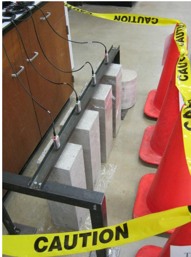
Figure 3-7 Shrinkage testing of beam specimens.
