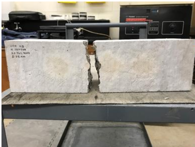
Figure D-7: Typical Upper Ridge Road NB conventional concrete specimen after flexural strength testing.
