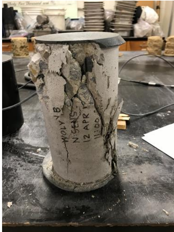
Figure D-2: Typical Wolverine Way NB TSMR specimen after compressive strength testing.
