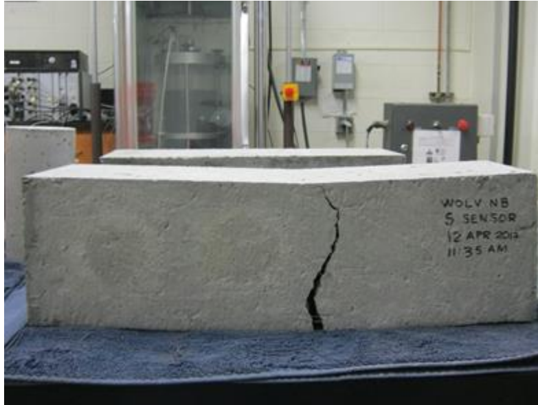
Figure D-6: Typical Wolverine Way NB TSMR specimen after flexural strength testing.
