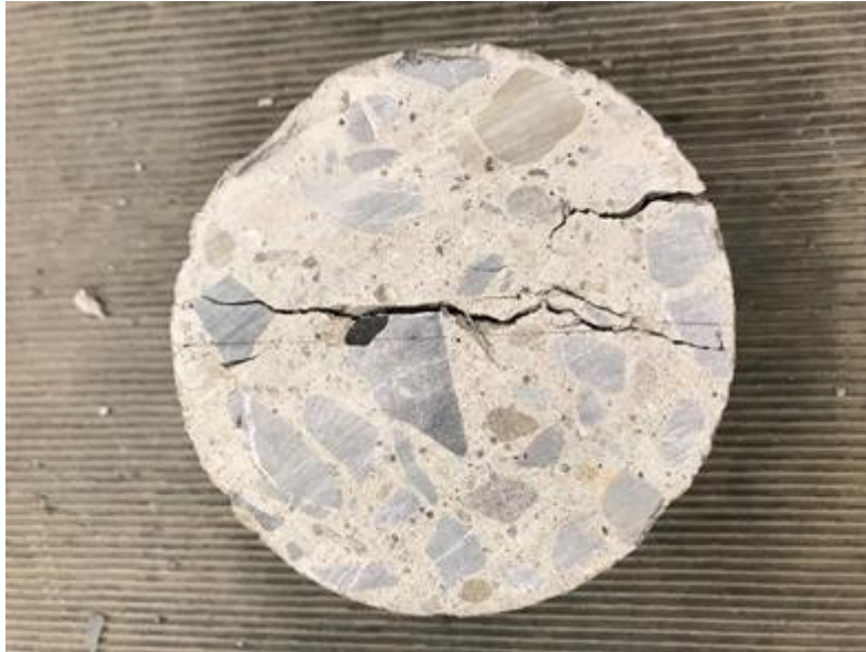
Figure D-10: Typical Wolverine Way NB TSMR specimen after splitting tensile strength testing.
