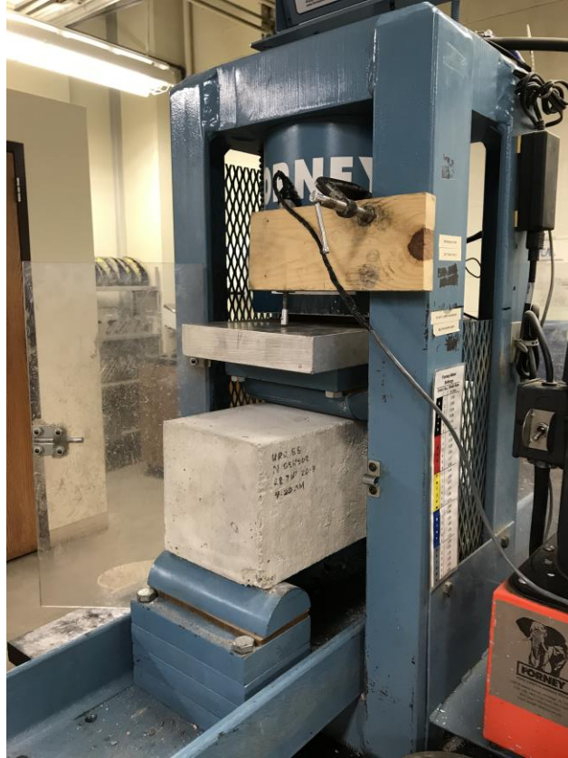
Figure 3-10 Flexural strength testing.
