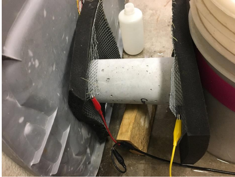
Figure 3-8 Electrical impedance testing of a cylindrical specimen.
