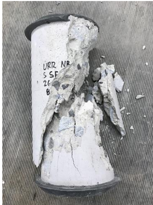
Figure D-3: Typical Upper Ridge Road NB conventional concrete specimen after compressive strength testing.
