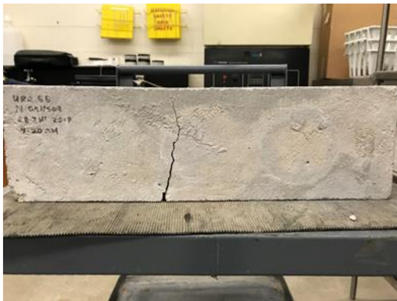
Figure D-5: Typical Upper Ridge Road SB TSMR specimen after flexural strength testing.
