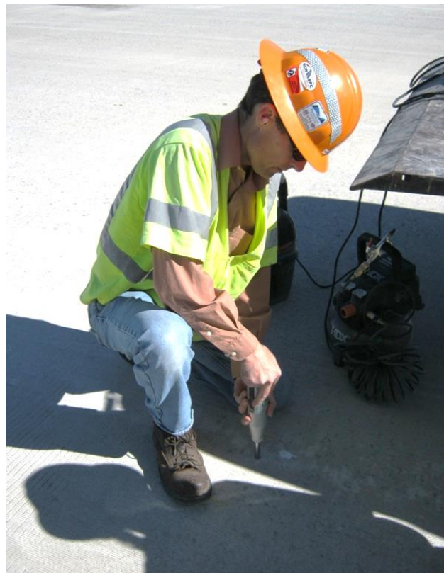
Figure 3-12 Schmidt rebound hammer testing.
