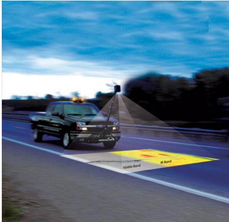
Figure 2-18 Vehicle-mounted infrared thermography scanning (Ruohonen 2013).
