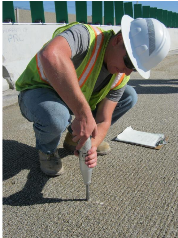
Figure 2-26 Schmidt rebound hammer testing.
