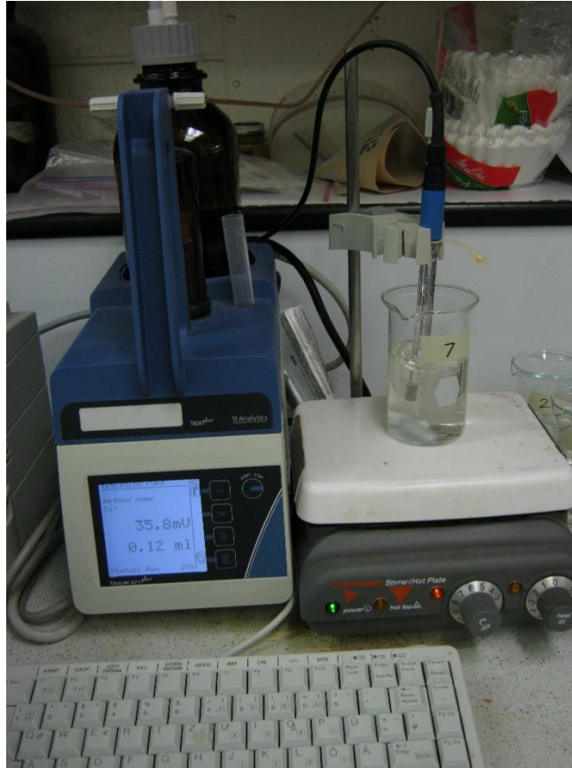
Figure 2-3 Chloride concentration testing.
