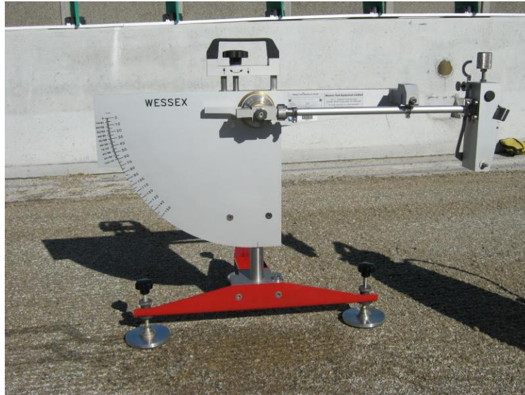
Figure 2-28 Skid resistance testing using the BPT apparatus.
