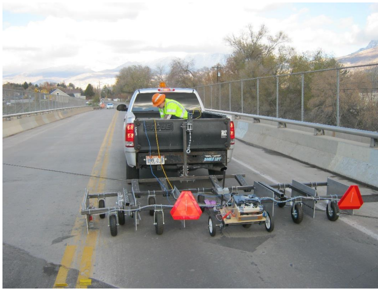
Figure 2-15 Mallet-based multi-channel impact-echo scanner.
