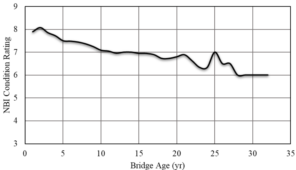
Figure 3-6: Average deterioration curve for bridge decks with early application of a bituminous overlay in Region 2.
