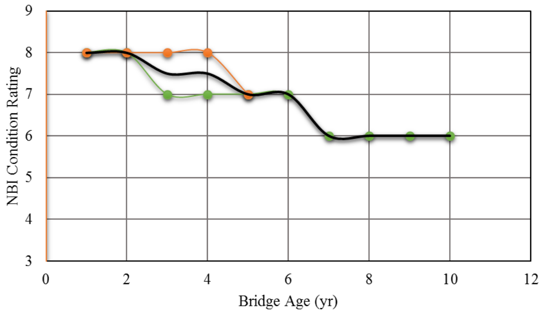
Figure B-18: Individual deterioration curves and average curve aligned by deck construction time for bridge decks with early application of latex-modified concrete in Region 4.
