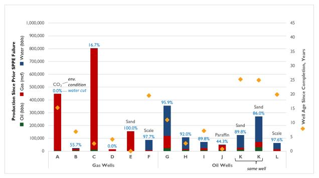
Figure 37: Production from Wells with Repeated Failures, 2020
