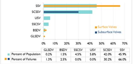
**NOTE**: Includes 159 total failures. Excludes 13 failures of subsurface safety valves identified in OGOR-A data where it could not be confirmed whether they were SCSSVs or SSCSVs.
