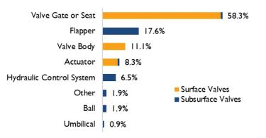
**NOTE**: Percentage is of 108 failures where the failed component was known to BTS. Total exceeds 100 percent because more than one component may be reported for a single event.
