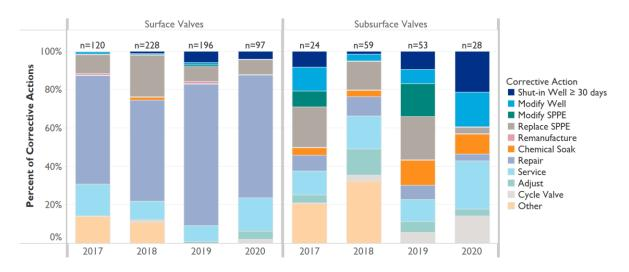
Figure 30: Reported Corrective Actions, 2017-2020 (SafeOCS Failures Only)
