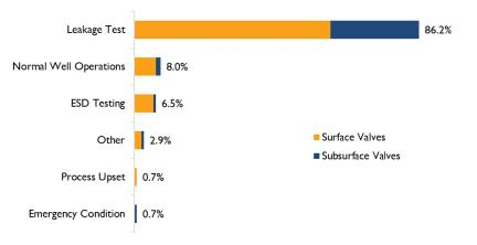
**KEY:** ESD—emergency shutdown. **NOTE:** Percentage is of 138 failures where the detection method was known to BTS. Total exceeds 100 percent because more than one detection method may be reported for a single event. **SOURCE:** U.S. Department of Transportation, Bureau of Transportation Statistics, SafeOCS Program.
