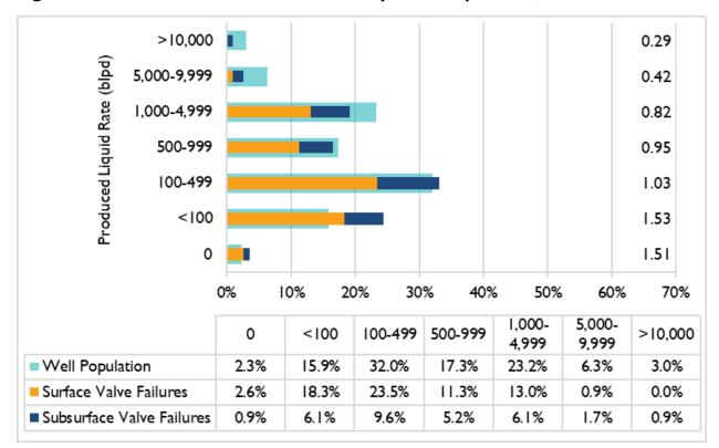
Figure 23: SPPE Failures and Active Wells by Total Liquid Rate, 2020
