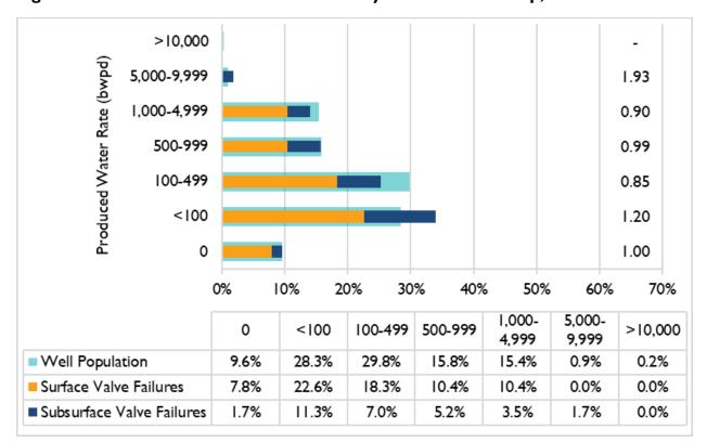
Figure 21: SPPE Failures and Active Wells by Water Rate Group, 2020
