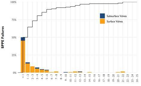
Figure 35: Time to Failure, 2017-2020
