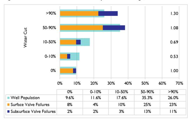
Figure 22: SPPE Failures and Active Wells by Water Cut Range, 2020
