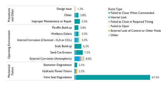
Figure 32: Factors Contributing to Equipment Failures, 2020
