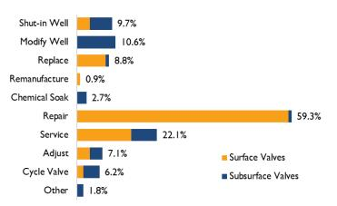
**NOTE:** Percentage is of 113 failures where the corrective action was known to BTS. Total exceeds 100 percent because more than one corrective action may be reported for a single event. Corrective actions are listed from higher to lower degree of intervention.
