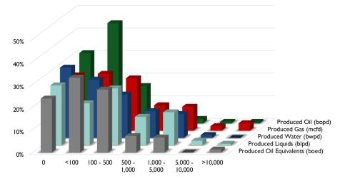
Figure 16: Failures Grouped by Well Fluid Rate Ranges, 2020
