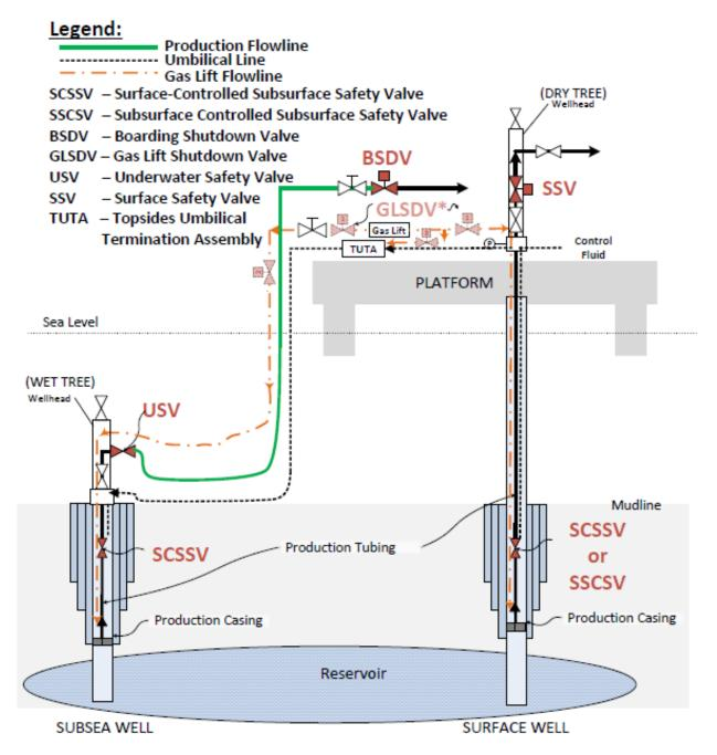
**NOTE:** GLSDVs for subsea wells may be installed in 1 of 3 alternate locations as described in 30 CFR 250.873: (1) Horizontal valve on gas lift supply line within 10 feet of the platform edge; (2) Vertical valve in gas lift supply line riser run within 10 feet above the first accessible working deck (excluding the boat landing and splash zone); (3) Gas lift supply via umbilical within 10 feet of the TUTA.
