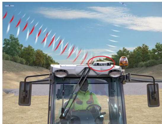
Figure 4. Global Positioning System Antenna
