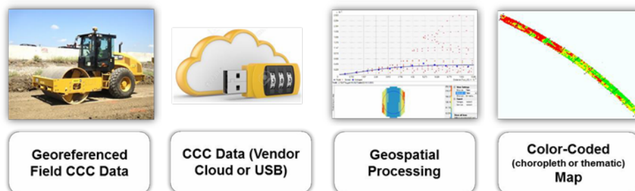
Figure 9. Process of Collecting IC Data and Generating the Compaction Quality Map
