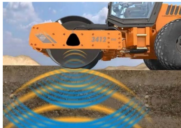
Figure 8. Vibration Response from Soil Layers
