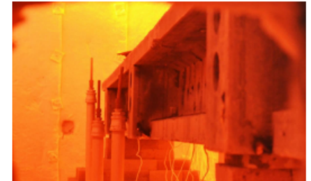
Concrete beams prestressed with CFRP strands were subjected to fire/loading tests to evaluate their fire endurance.
