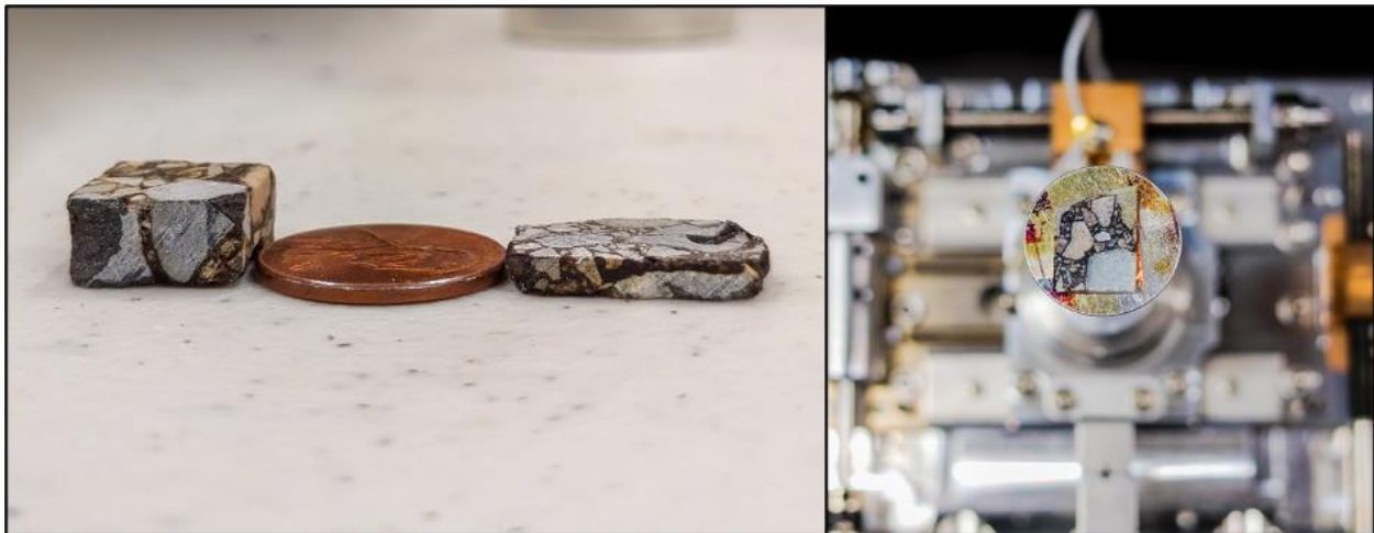
Figure 6-4 Sample for SEM-EDX Analysis
