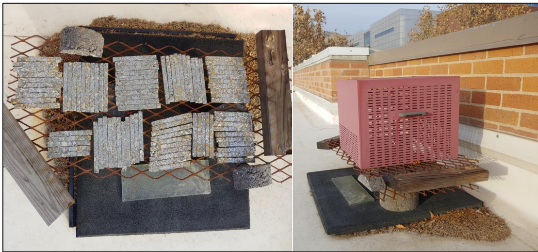
Figure 6-1 Picture of Beams Placed on the Roof to Evaluate Natural Aging.
