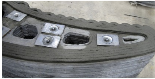
b) Example of 3D printed “wall” with voids for reinforcing steel.
