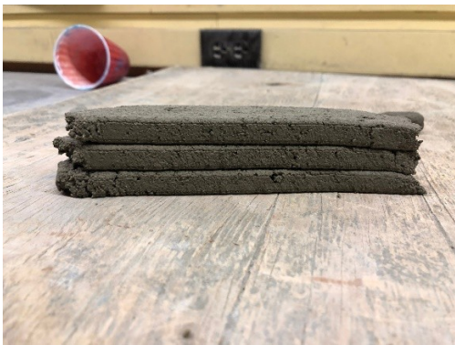
Figure 3.8 0.30 W/C ratio with Walocel
