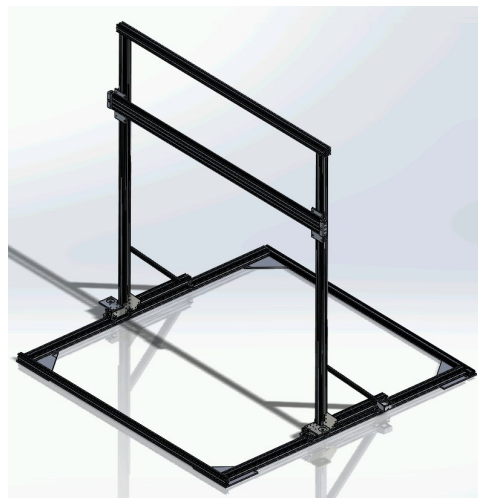
Figure 4.1: SolidWorks rendering of the gantry machine; the stepper motors and drive mechanisms are not pictured.
