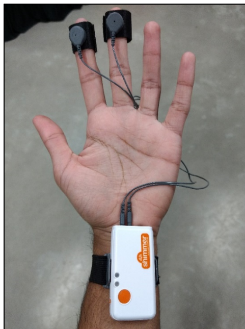
Figure 3.1 Shimmer3 GSR+ sensors (shown attached to the index and middle finger) send data to a host computer through the wireless transmitter (shown attached to the wrist) in real time
