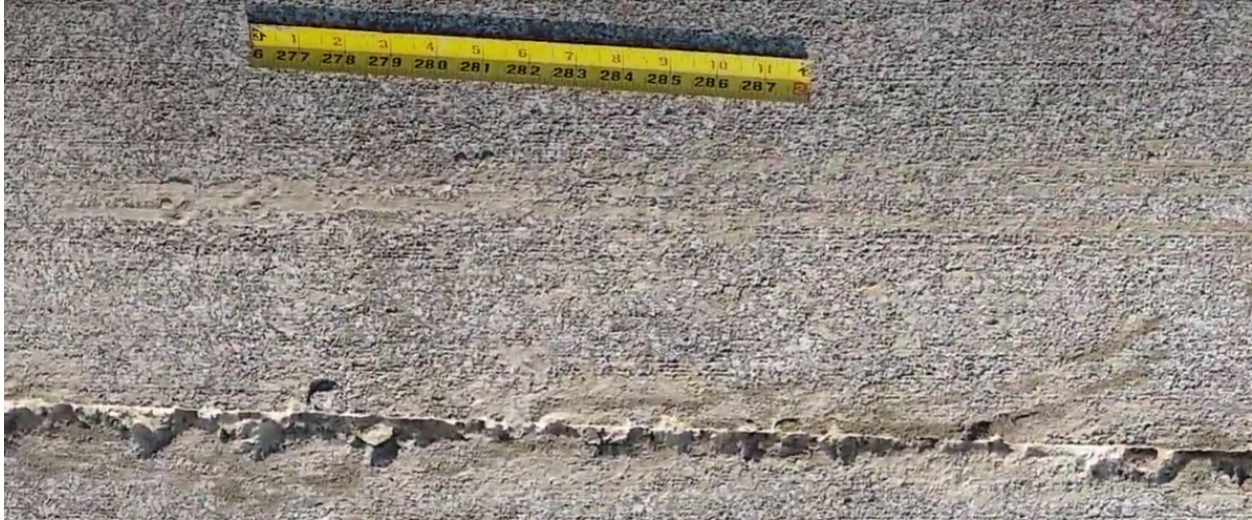
C. HVFAC mix: Saw cut after 6 hours 20 minutes
