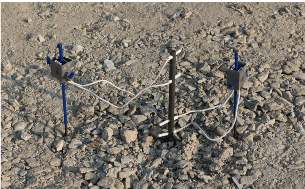
B. Close-up photograph of the wireless thermal sensors
