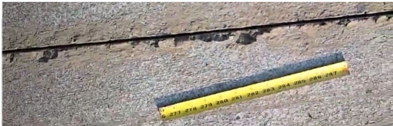
B. HVFAC mix: Saw cut after 5 hours 35 minutes
